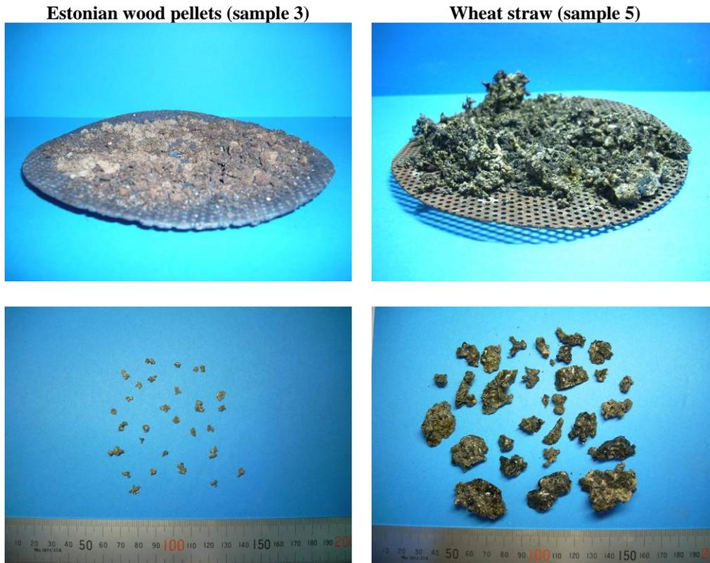
Figure 8: Grate with remaining ash and sieved ash and slag-particles ( $> 2.5$  mm) after test in the Slagging Analyser with Estonian wood pellets (sample 3) and wheat straw (sample 5).
