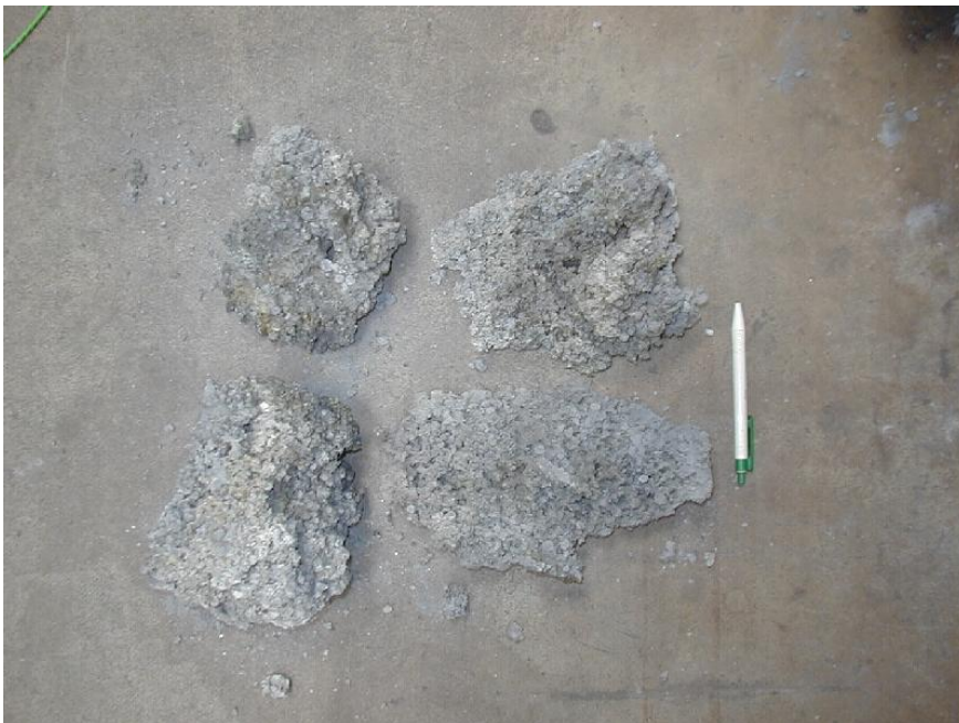
Picture 8-3. Typical slag formation. Slag from R3.
