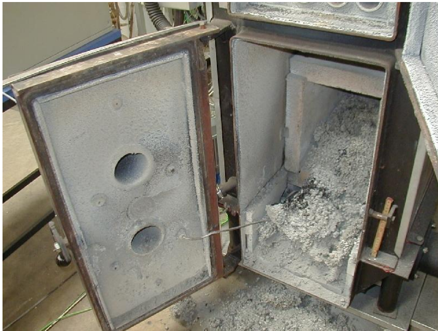
Picture 8-14. The picture was taken shortly after shut down. There was a lot of slag which the ash screw had not been able to remove. The combustion chamber was also heavily fouled in spite of the fact that the test duration was very short.
