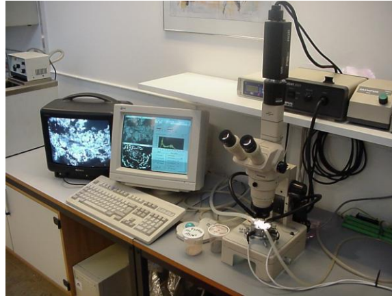
Picture 9-1. Equipment for the MAF Method. A few micrograms of a sample of homogenized (laboratory prepared) ash is placed on a sapphire disc (7 mm in diameter), which is inserted in a gas tight heating stage below a microscope. Nitrogen is used as atmosphere. The microscope is focused on a random part of the sample and the magnification is set at about 100 X.
