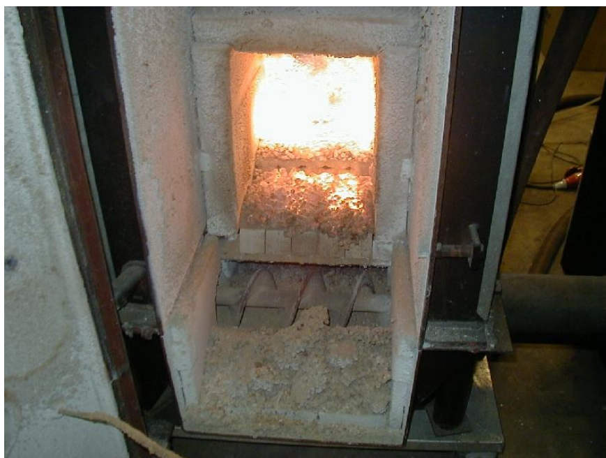
Picture 8-21. The picture was taken shortly before shut down. There was a small quantity of slag in the ash, but it was crumbly and therefore easily removed by the ash screw. The combustion chamber was slightly fouled.
