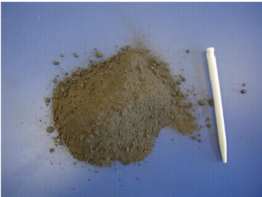
Picture 8-5. Typical ash consistency when there is no slag. Ash from R8.
