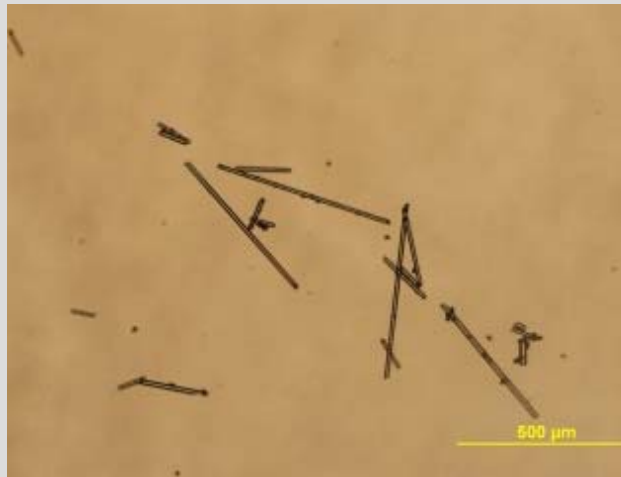
Glasfibre (500 \mu\text{m} x 10 \mu\text{m} ) Varmedæmning
