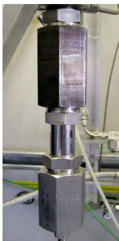
Figure 1: High-pressure 316 stainless steel reactor with total internal volume of 54 ml.
