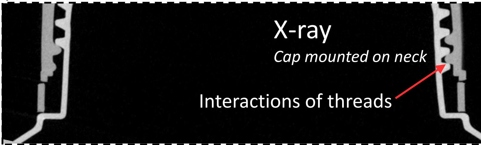
Cross-section of the polymer cap and neck
