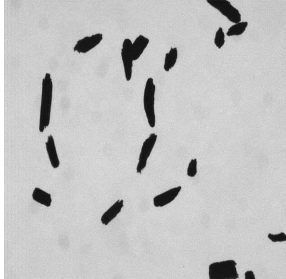
Figure 17: Milled torrefied wood chips (280°C)
