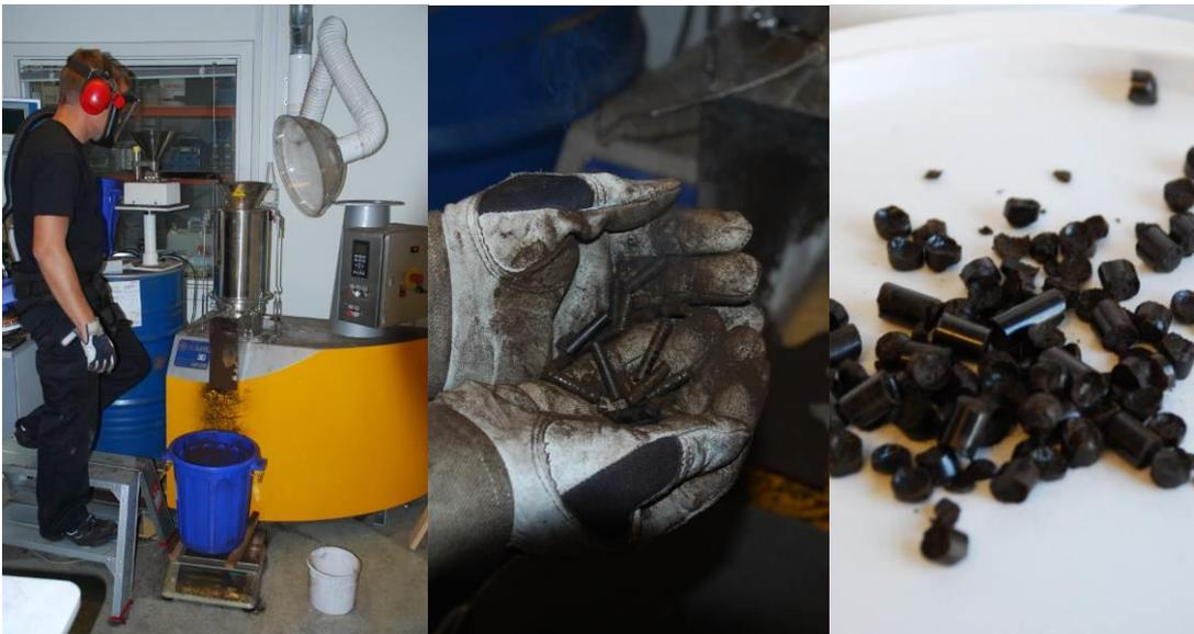
Figure 18: The Kahl Pellet mill during pelletisation of torrefied wood (a) the mill , (b) pellets from torrefied beech wood, (c) short pellets from torrefied pine with addition of 2 % rape seed oil
