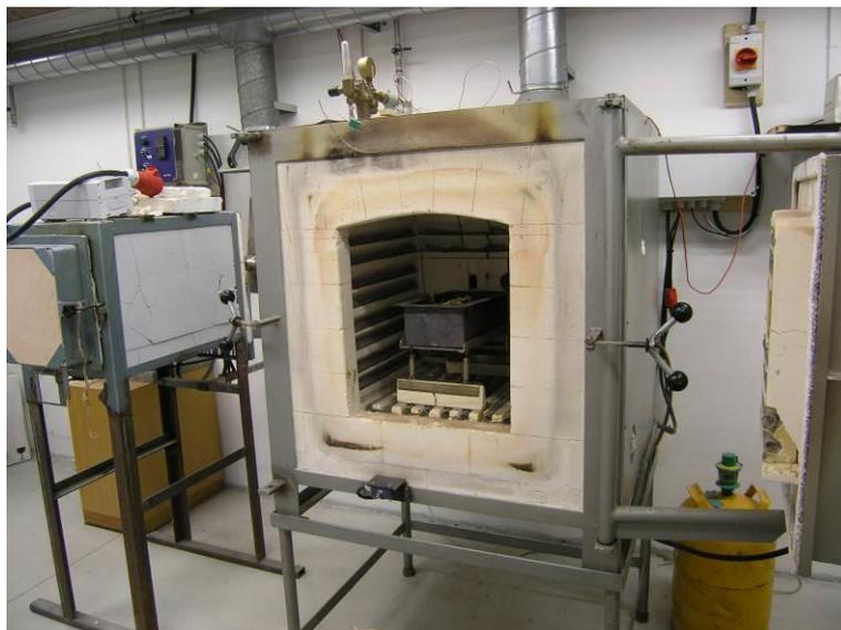
Figure 2: The pyro-oven (Lyngbyovnen of type S 90, 3 × 380 V, 9 kW)
