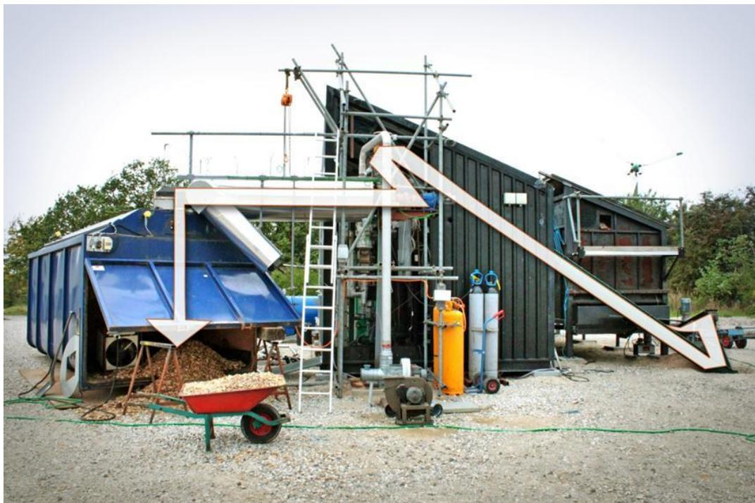
Figure 3: Picture of the torrefaction test unit at Risø/DTU
