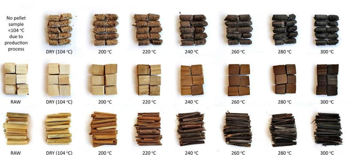
Figure 12: Samples from torrefaction test in the pyro oven (wood pellets, wood and straw)
