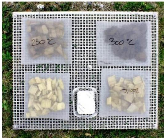
Figure 6: Experimental setup for long term outdoor test of water uptake. Picture was taken top down.
