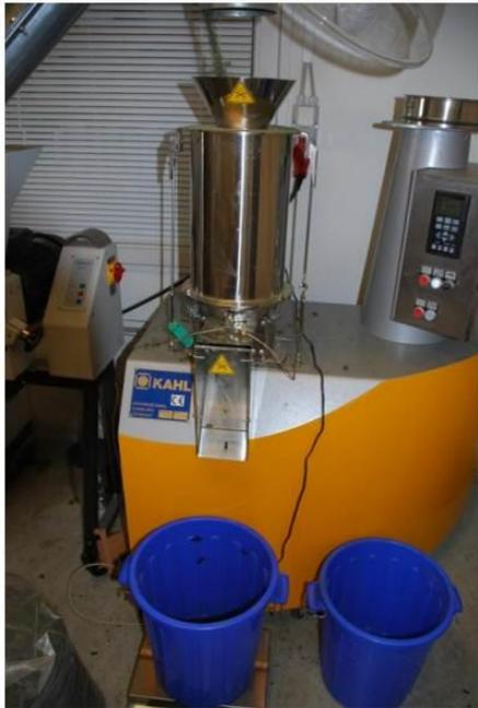
Figure 7: The flat die bench scale pellet mill (~5-10 kg/h)
