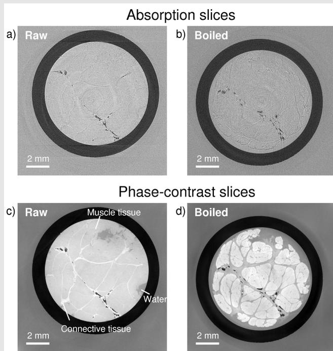
Panels a) - b) show absorption tomographic slices of a piece raw and boiled bovine meat, respectively. By comparing with the phase-contrast slices in panels c) and d), it is seen that the contrast between muscle tissue, connective tissue and water is improved vastly. Using phase-contrast it is seen that the connective tissue has absorbed water during heating whereas the muscle protein has lost water.
