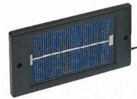
Figure 8 Solar cell used as light logger
