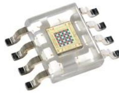
Figure 41 TAOS TCS230 color sensor
