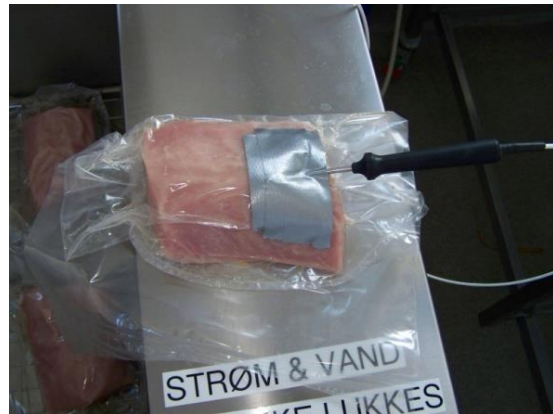
Fig.3 The temperature dummy to monitor the core temperature
