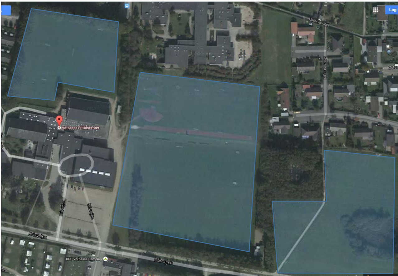
Figure 1: Vorbasse Fritid Center integrated sports facility and kindergarten can be seen left in the picture with surrounding areas and suggested potential areas for collecting thermal heat with a heat pump (the area far to the right being optional).
