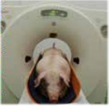
General Electric HiSpeed Zx/i 140 kV, 145 mA, 512x512 matrix. Axial 10 mm-thick slices every 10 mm (7 mm-thick every 7 mm in 30 kg pigs).
