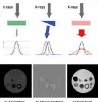
Figure 2. GBI modalities capturing attenuation, refraction and scattering.
