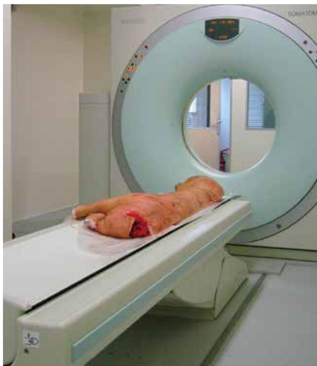
**Figure 1a.** CT scanning a pig half-carcass.
