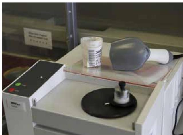
**Figure 1.** NIRFlex N-500 (Büchi Labortechnik AG, Flawil, Suisse) equipped with a glass measuring cell of 3.4 cm diameter x 2.5 cm with a metallic accessory placed on the surface of the fat sample for homogeneous pressure on the sample.
