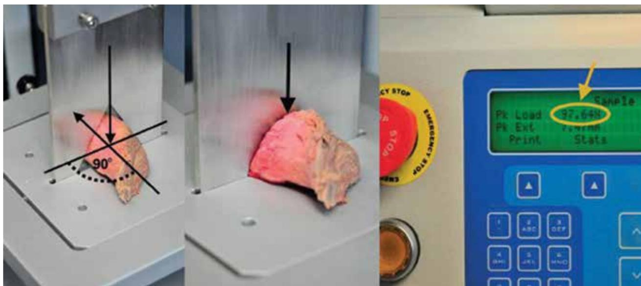
**Figure 4.** Steps in the determination of Warner-Bratzler shear force with a texturometer.
