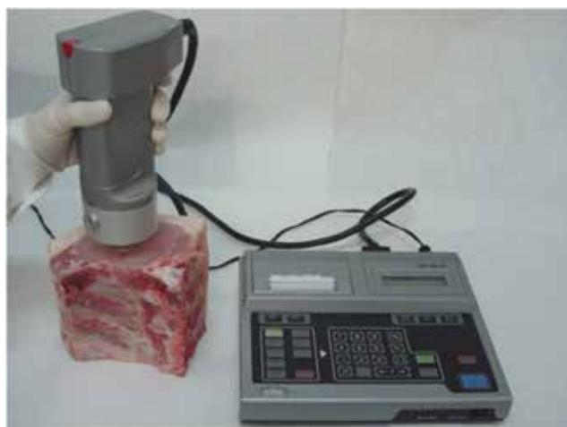
**Figure 3.** Determination of L\*, a\* and b\* colour parameters with a Minolta colorimeter.
