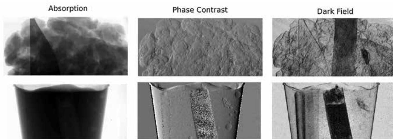
**Figure 2:** The results from GBI of organic foreign bodies placed in food products. Top: Minced meat with broken glass (left), 4 layers of paper (middle) and ladybug (right). Bottom: Sour cream with 8 layers of paper (left), a cigarette butt (middle) and a fly (right). Reprinted from (Nielsen *et al.* 2013)
