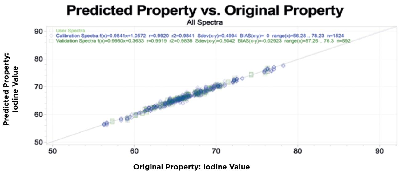
**Figure 3.** NIRS predictions for iodine value in calibration and validation samples, *versus* reference values. Iodine value was calculated based on the monounsaturated and polyunsaturated fatty acid methylester level.
