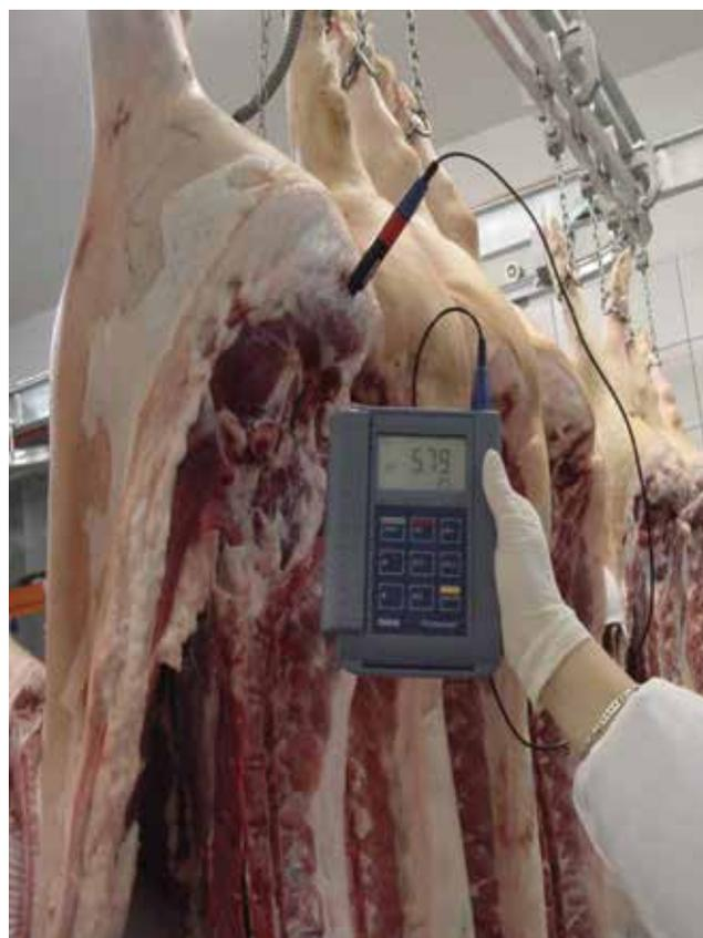
**Figure 1.** Measure of pH on muscle *Semimembranosus* at 24 h post mortem.
