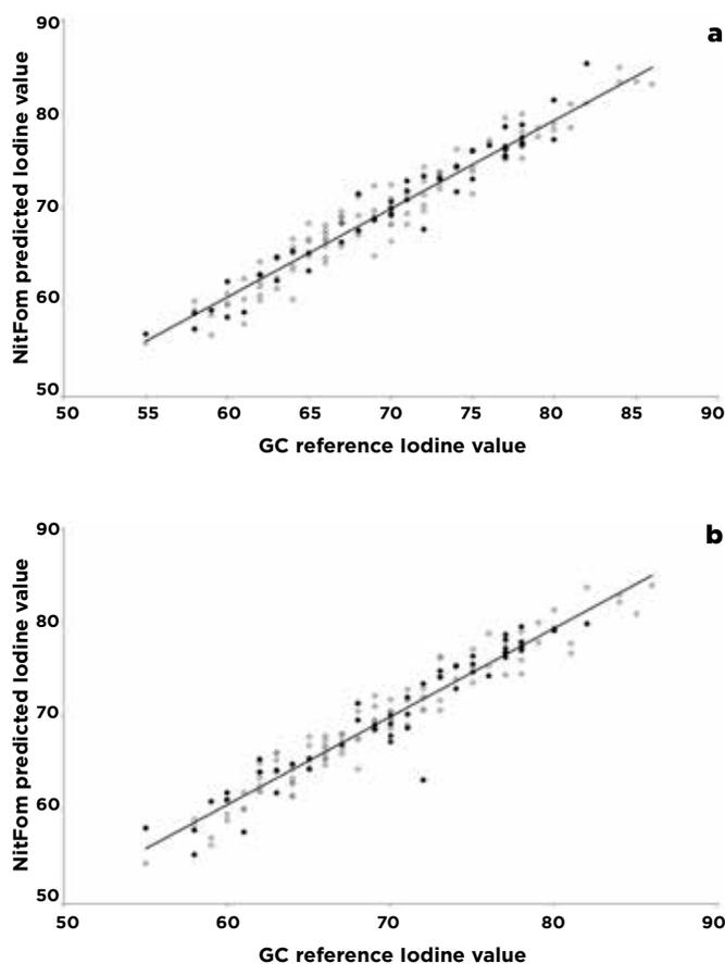
**Figure 1:** Relationship between GC reference and NitFom predicted iodine value in hot (a) and cold (b) fat samples. Open symbols represent the calibration data set (n=100) and filled symbols represent the validation data set (n=50).
