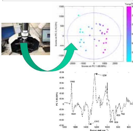
Figure 1. PCA of Raman spectra from *longissimus thoracis* muscle cooked at 50 – 80 °C for 2h then stored at 4 °C for 4 days. PC-score plot coloured according to cooking temperature (top) and PC-loadings plot for PC-1 (bottom). (n=32)
