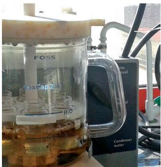
Figure 1: Acid hydrolysis process.
