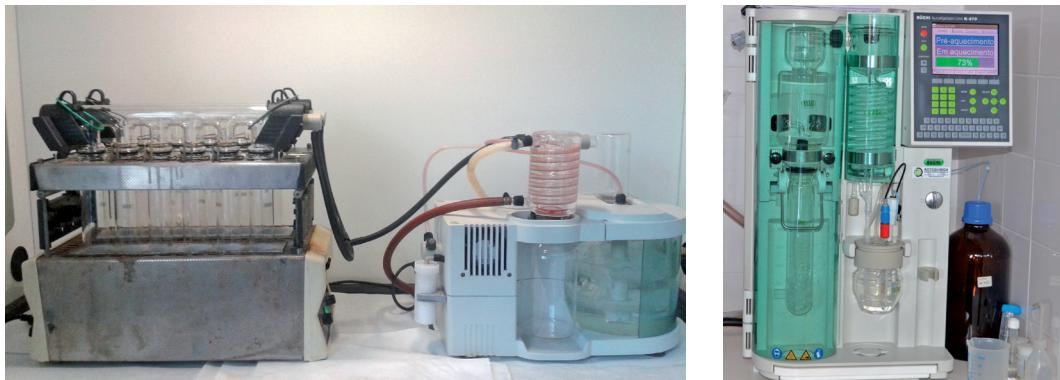
Figure 1: Digestion (left) and distillation (right) process to determine protein content.
