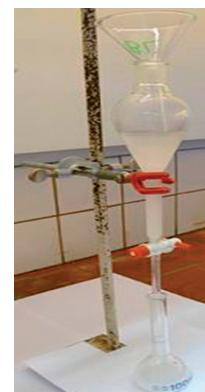
**Figure 3:** Two phases separation of the solvent mixture.
