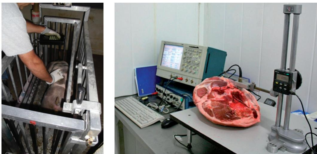
Figure 9: Ultrasound measurement of fat in live pigs (left) and ham (right).
