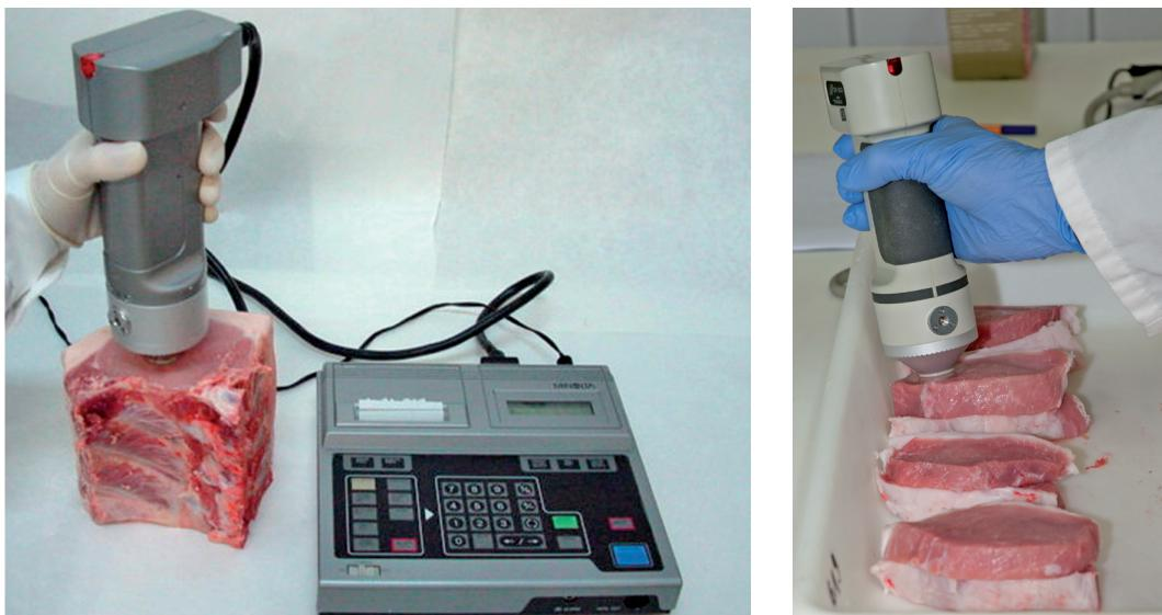
Figure 3: Determination of L\*, a\* and b\* colour parameters with a Minolta chromameter.
