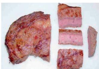
Figure 8: SSF slice prepared for shearing. From Shackelford et al. (2009).
