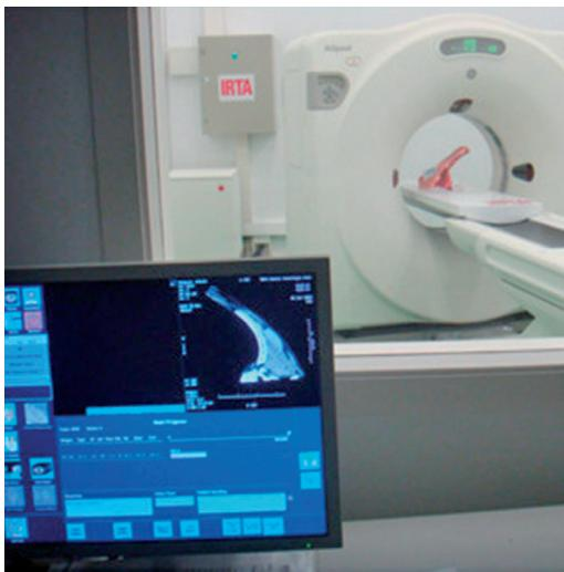
Figure 2: Beef rib measured with a computed tomography equipment.
