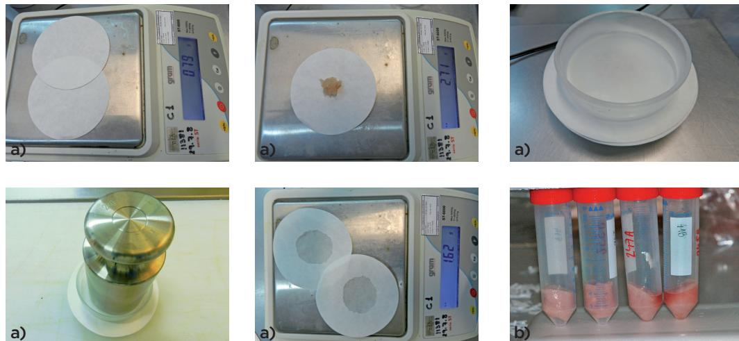
Figure 4: Determination of WHC using a) filter paper press methods (in chicken meat) and b) high-speed centrifugation (in pork loin).
