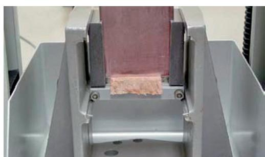
Figure 12: SSF shearing on a universal testing machine. From Shackelford et al. (2009).
