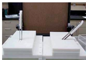
Figure 9: 90° and 45° slice boxes. From Shackelford et al. (2009).
