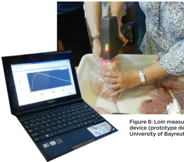
Figure 8: Loin measured with a portable RAMAN device (prototype device of Heinrich Schmidt, University of Bayreuth, Germany).
