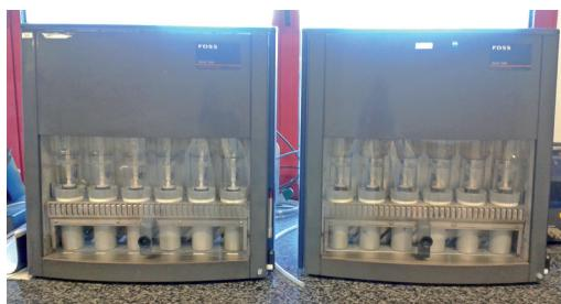
Figure 3: Equipment used to determine fat content with Soxhlet method.
