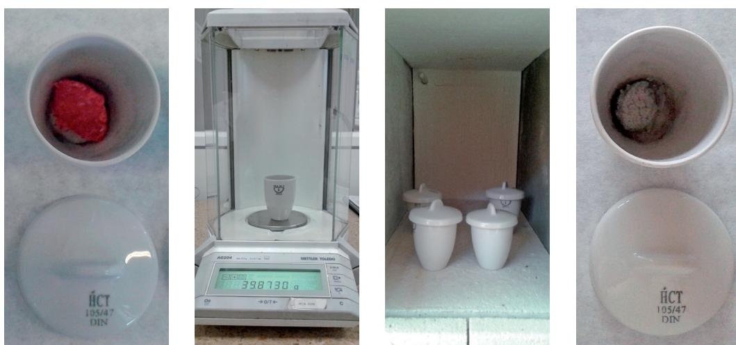
Figure 4: Ash evaluation process, from left to right, fresh sample, weighing, muffle oven and ash.
