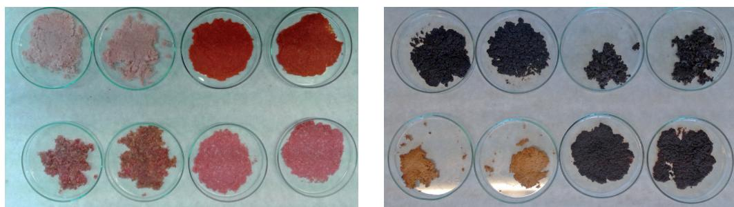
Figure 2: Meat before and after drying to obtain the moisture content.
