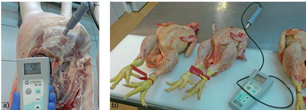
Figure 2: Measurement of pH a) in pig muscle *semimembranosus* and b) in chicken breast (*pectoralis major*).
