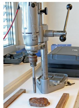
Figure 2: Electric drill press with cork borer attached.
