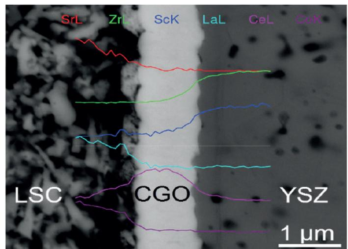
**Figure 1:** Scanning electron micrograph and energy-dispersive X-ray (EDS) linescan across the CGO barrier obtained after fuel cell operation. EDS show the chemical composition across the barrier. Note the top red line shows the Sr content to be high in the LSC cathode but the CGO barrier successfully blocks Sr diffusion to the Sc-doped YSZ electrolyte.
