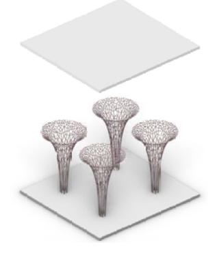
20 thick elements 3D printed with extra fine nozzle optimized to save material
