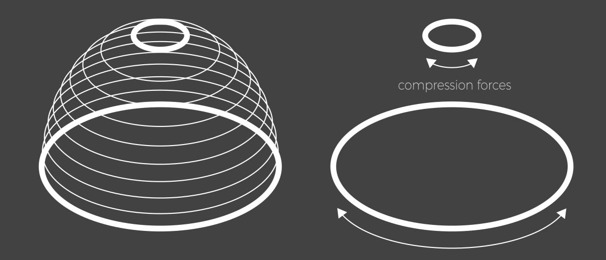
The dome works only in compression. The steeper the angle, the smaller the radius.
