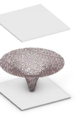
One supportive roof-column element Optimized to save material
