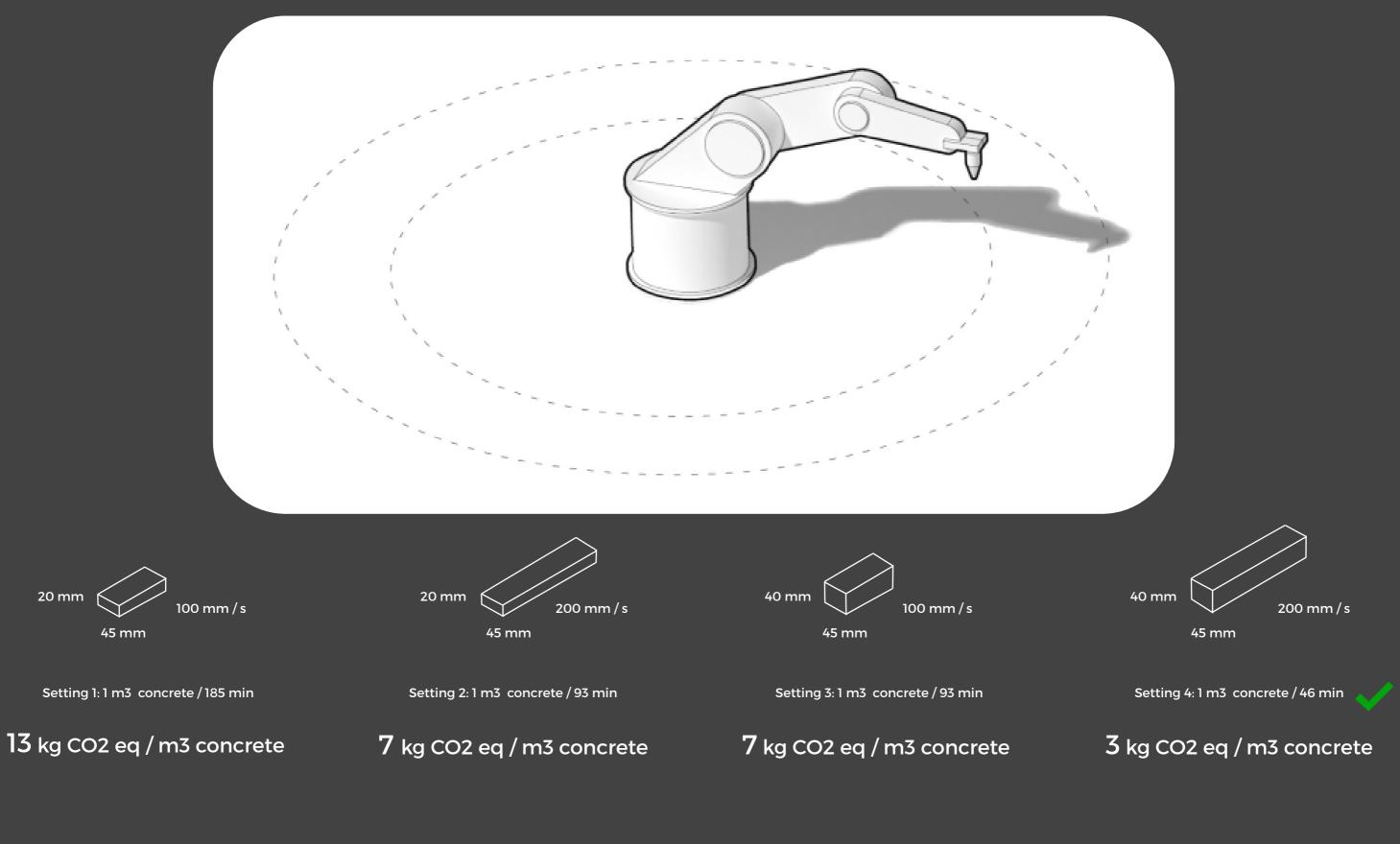
Printing fast uses more energy, but the robot has to run for a shorter period of time - resulting in the lowest carbon emissions!
