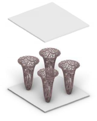
40 mil thick elements 3D printed with fine nozzle Optimized to save material
