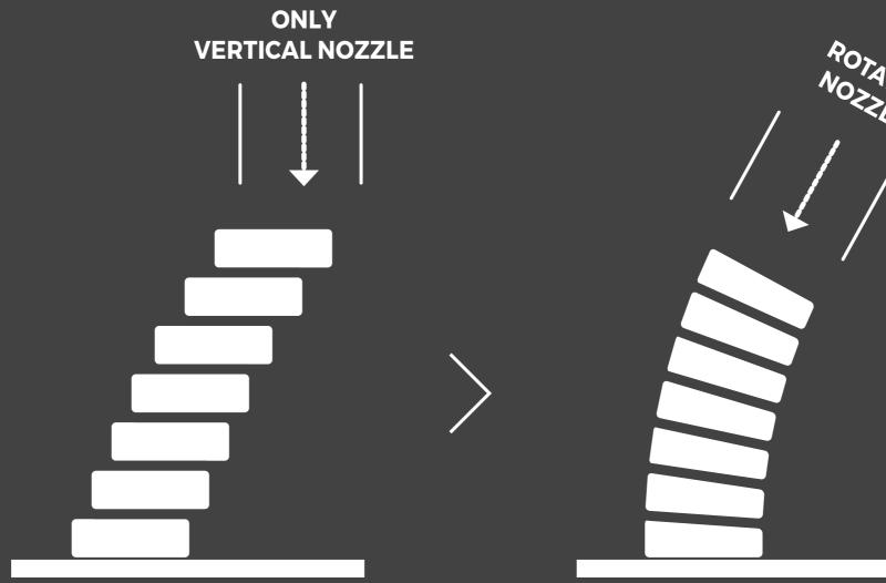
It is possible to consider the rotation of nozzle during the print. That could make the wall more structural, because each layer would adhere better to the layer below.
