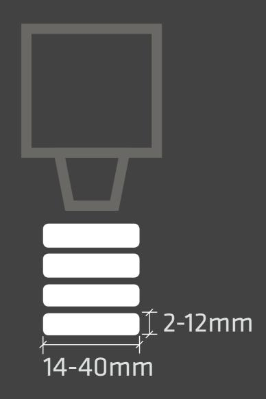
Typically, the maximum width for a layer is between 14mm and 40mm and the maximum layer height varies between 2mm and 12mm. It also varies based on different types of nozzles.
