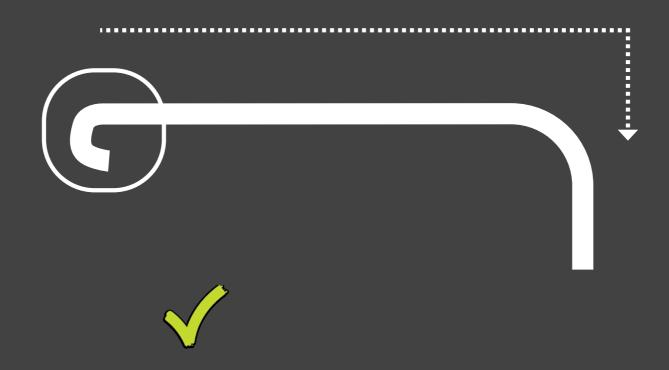
It is recommended to hide the starting point of the print or to integrate it within the structure.
