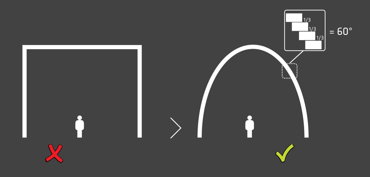
Due to the nature of the extrusion technique, it is technically not possible to print horizontal members without scaffolding or other considerations. Maximum cantilever is 1/3 of each layer which is about 60 degree angle.
