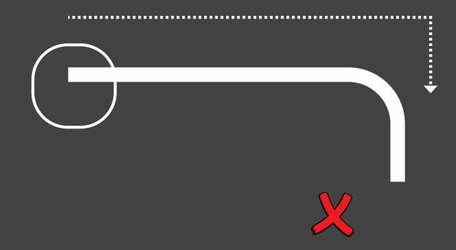
At the beginning of each layer's extrusion, it is difficult to control the ejection and precision.
