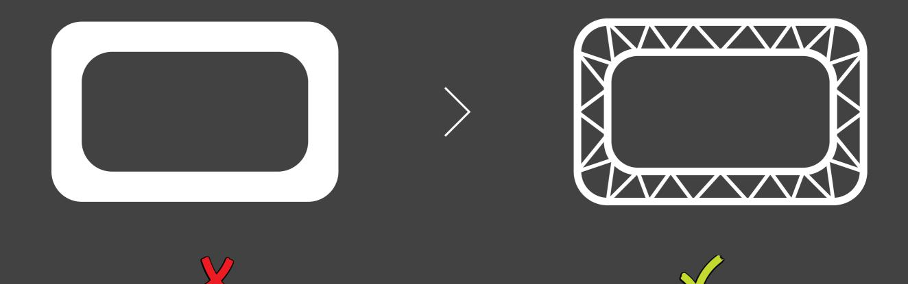
To be structurally stable and economically efficient, it is better to print a double wall instead of one thick wall. It saves material and the cavity space can be used for structure, insulation, piping, and perhaps even program.
