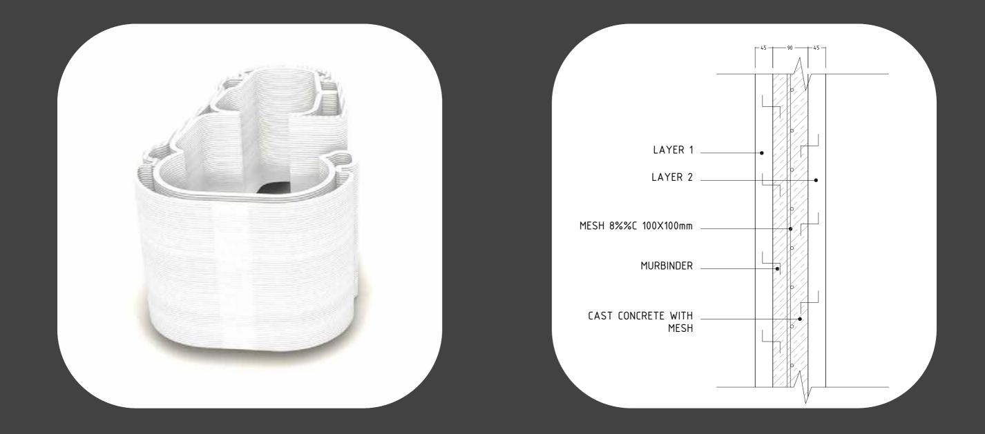
4 types of insulation are being considered for the cavities inside the walls: light weight concrete, EPS, blown-in cellulose fibre insulation from recycled paper, and blown-in wood fibre insulation. A wall section is composed of two layers of 3D printed concrete, each 45 mm wide and a cavity of 90 mm for insulation
