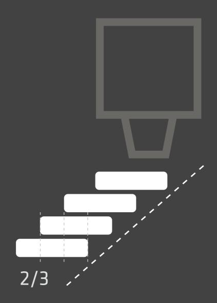
The maximum cantilever is 2/3 of each layer based on the most advanced technology by Sika AG.
