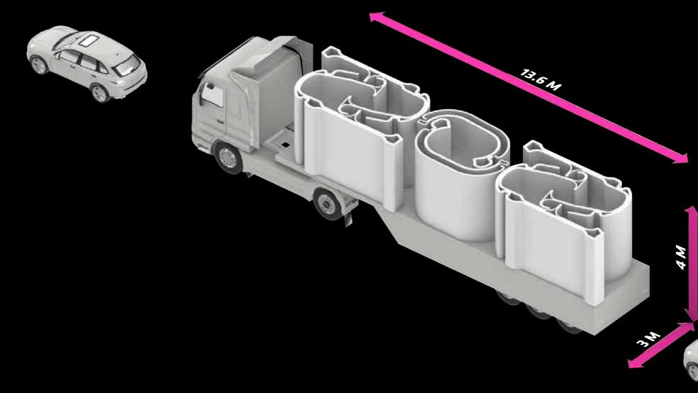
Taking in Consider The Constrains We are able to Transport **4 Units** at the Same Time Which Allows Us to Reduce the Time and Cost for the Transportation and Significant **Carbon Savings** In Transportation.
