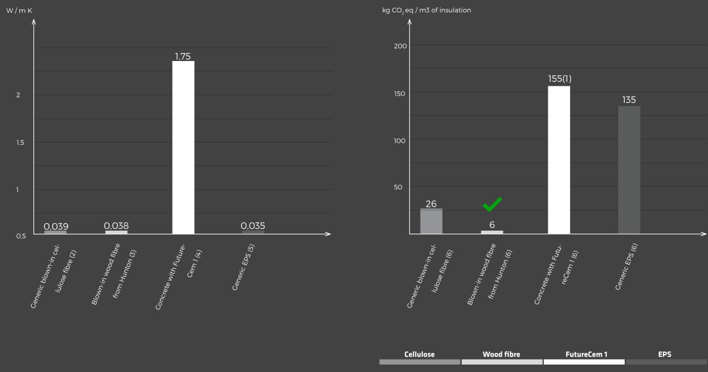
A high thermal conductivity means low insulation quality.
