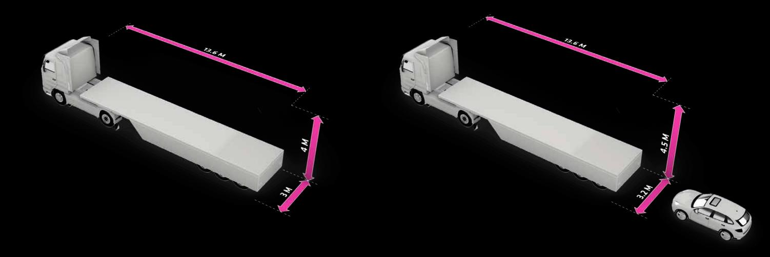
When it Comes to Transportation There is Some Off Site Constraints Like The Maximum Dimensions That we Can Build to Able to Transport is Important to Take in Considiration When Designing the Units to Reach the **Maximum Efficiency**
