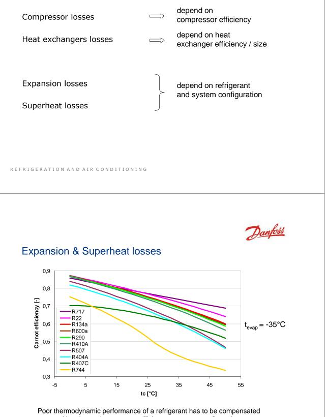
with enhanced component efficiency or system configuration
