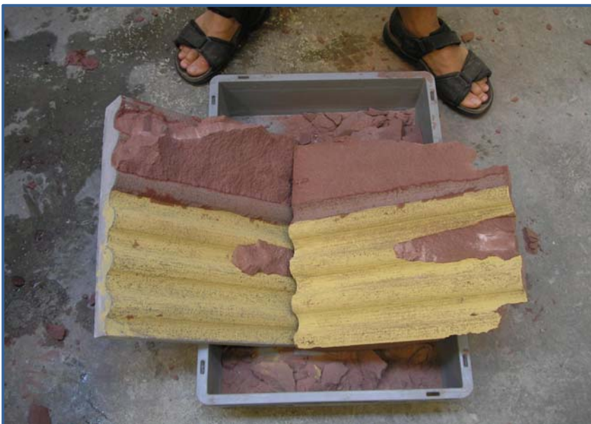
Fig. 21: De-molding was quite easy in the areas with the 'black' coating but it stuck to the concrete.
