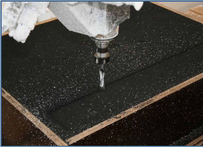
Fig. 22: Milling in moulding sand can be performed with very high speeds on both spindle and robot movement.
