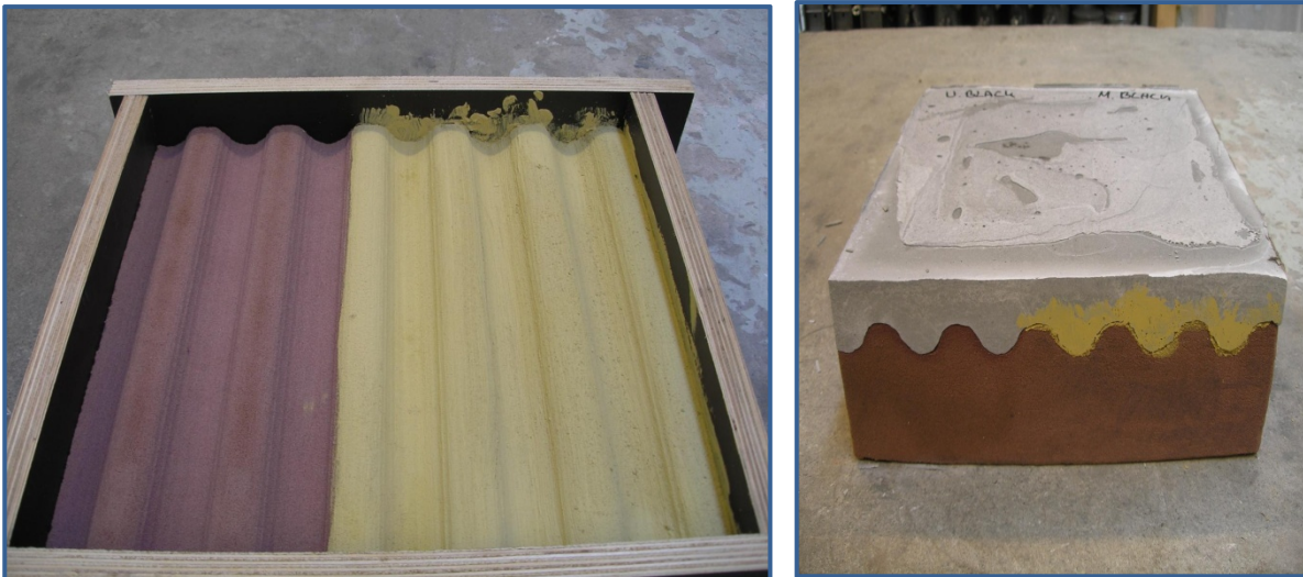
Fig. 20: Experiments with furan-sand where the one half of the mold was covered with 'black'.
