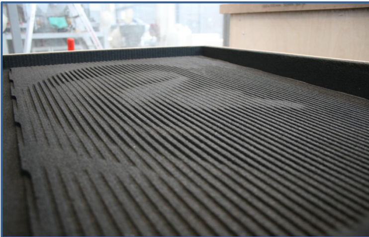
Fig. 24: Very fine details creating a 3D picture - milled in moulding sand without small pieces broken off.
