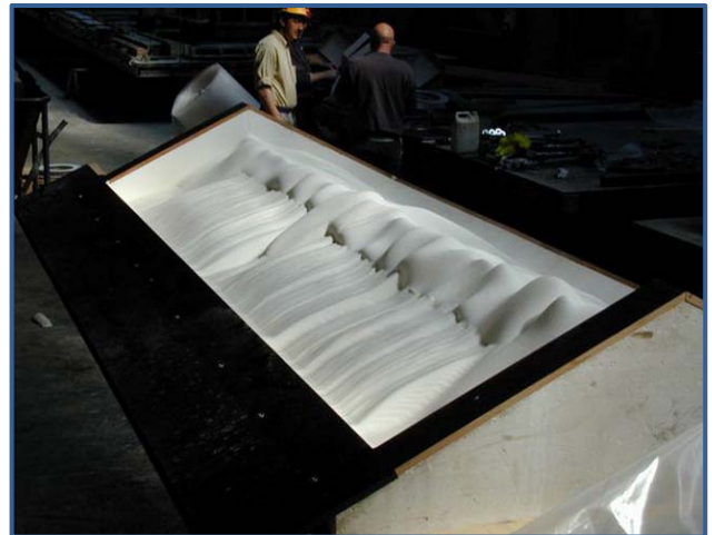
Fig. 29: Left: The robot mill out the polystyrene part for the formwork. Right: The parts brought together in the final formwork ready for the casting.
