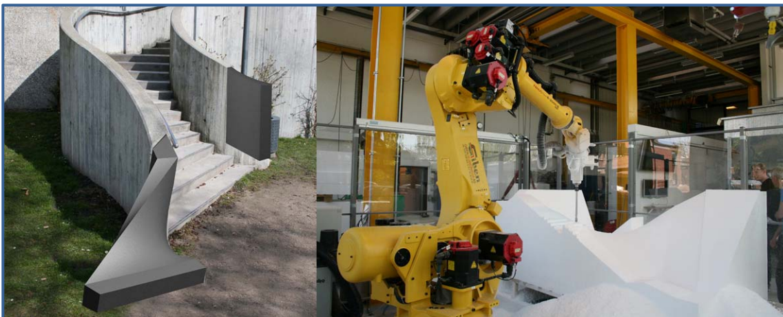
Fig. 25: On the left is a computer model of the concrete elements. On the right is the production of the moulds using robot technology at Danish Technological Institute.
