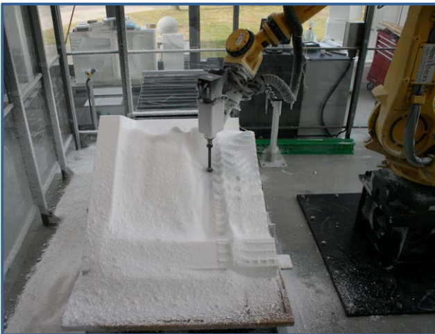
Fig. 29: Left: The robot mill out the polystyrene part for the formwork. Right: The parts brought together in the final formwork ready for the casting.
