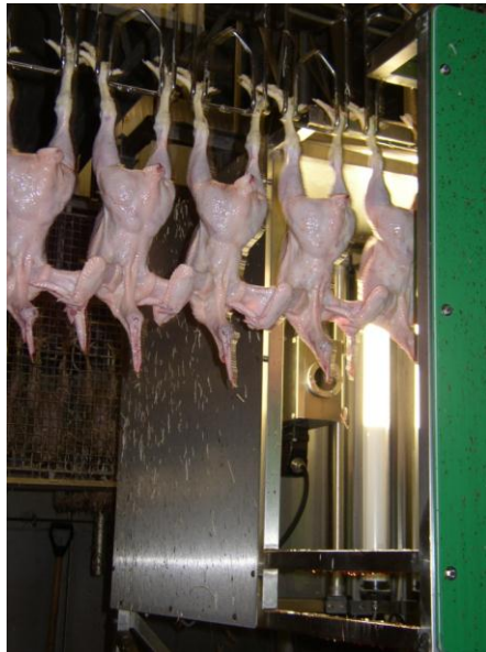
Picture 2. Box with camera, lamps and green back plate
