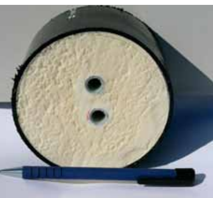
Twinrør i meget små dimensioner. Twin pipes in very small dimensions.
