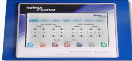
Outside weather compensation automatically adjusts the heating set point, so if the outside temperature rises the Spirax EasiHeat™ HTG will automatically lower its temperature output.
