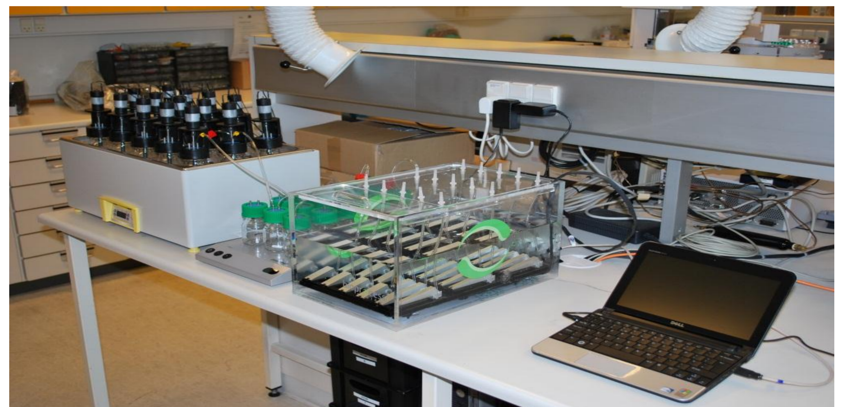
Figure 2: Experimental set-up of biomethane potential measurements.
