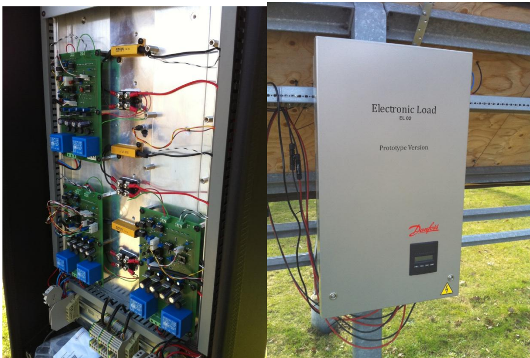
Electronic loads built by Danfoss Solar Inverters for the project
