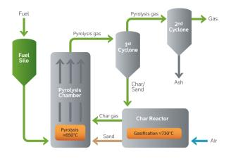
The Pyroneer gasifier typically consists of three main components; a pyrolysis chamber, a char reactor and a recirculating cyclone. A second cyclone is installed to remove particles from the produced gas.
