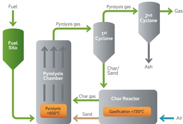
The Pyroneer gasifier typically consists of three main components; a pyrolysis chamber, a char reactor and a recirculating cyclone. A second cyclone is installed to remove particles from the produced gas.
