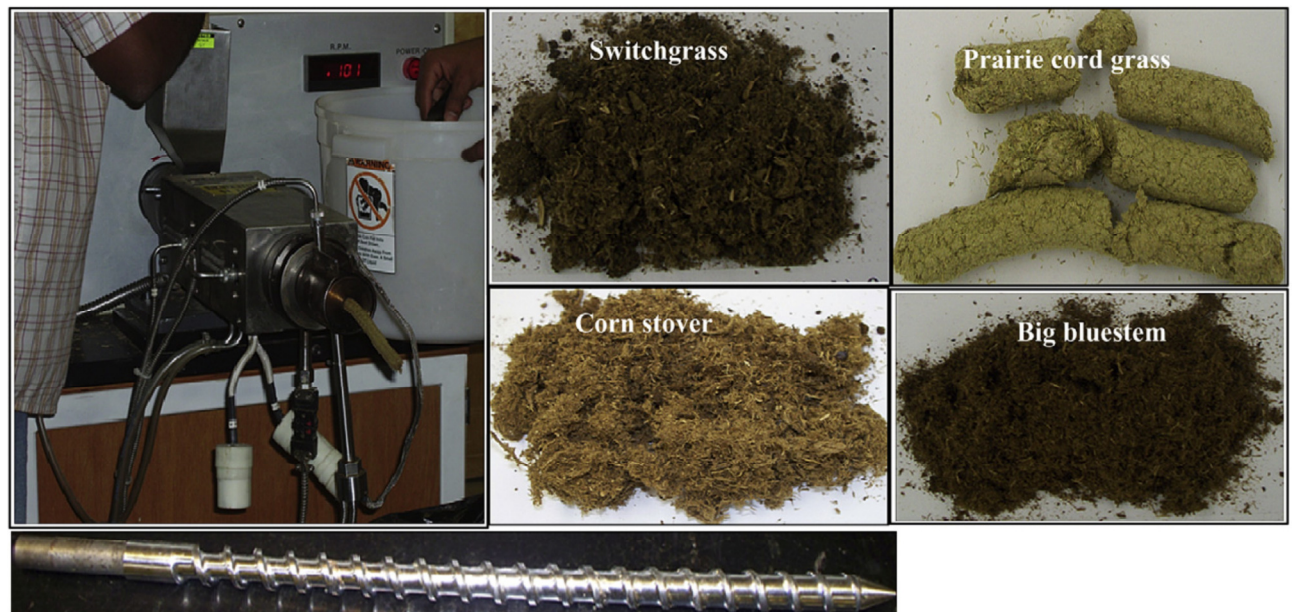
Figure 7. Laboartory single screw extruder and screw used for pre-treatment of different feedstocks (Karunanithy and Muthukumarappan, 2011a)
