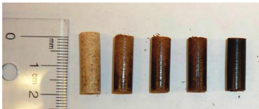
Fig. 1. Physical appearance of wood pellets treated at different steam explosion conditions. From left to right: untreated, 200°C for 5 min, 200°C for 10 min, 220°C for 5 min, and 220°C for 10 min (Lam et al. 2011).
