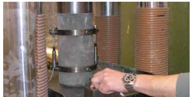
With the developed mix design it was possible to achieve two-day strengths of the concrete of approximately 10 MPa.
