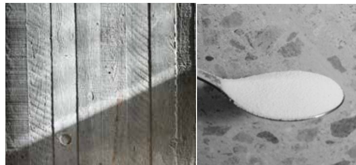
Adding Micronal ® - a type of Phase Changing Materials consisting of small capsules with paraffin - to concrete would theoretically increase the thermal mass.
