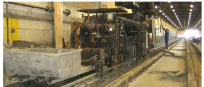
Hollow core decks were cast on top of the PCM-mortar tiles at the Spæncom A/S factory resulting in the final PCM-hollow core decks.
