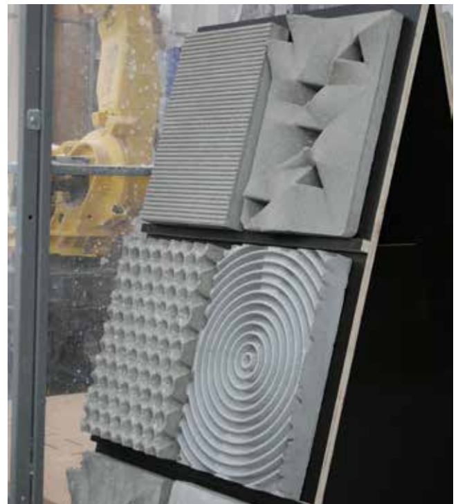
Concrete samples designed both to show aesthetic possibilities with profiled concrete surfaces and to test for acoustic properties.
