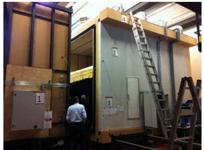
Hot-box for thermal measurements of hollow core decks at Aalborg University.
