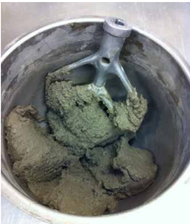
The concrete gets “sticky” and loose workability when PCM is added. This puts a limit on the amount of PCM which can be added.
