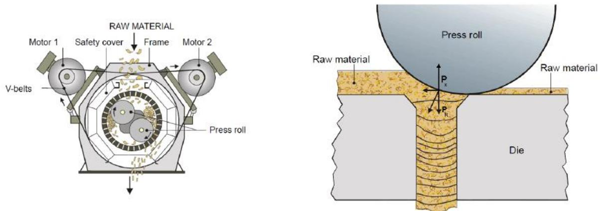
Figure 4. Illustration of the pelletizing process [11,12]
