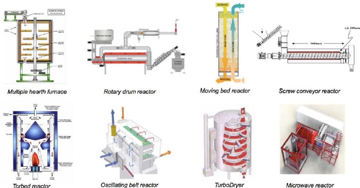
Figure 1. Different torrefaction technologies [7]
