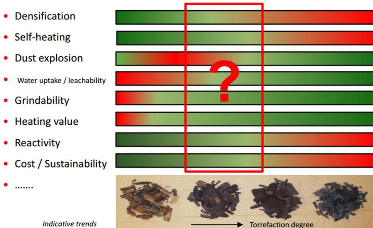
Figure 3. Impact of torrefaction degree on the fuel properties of torrefied biomass [10].
