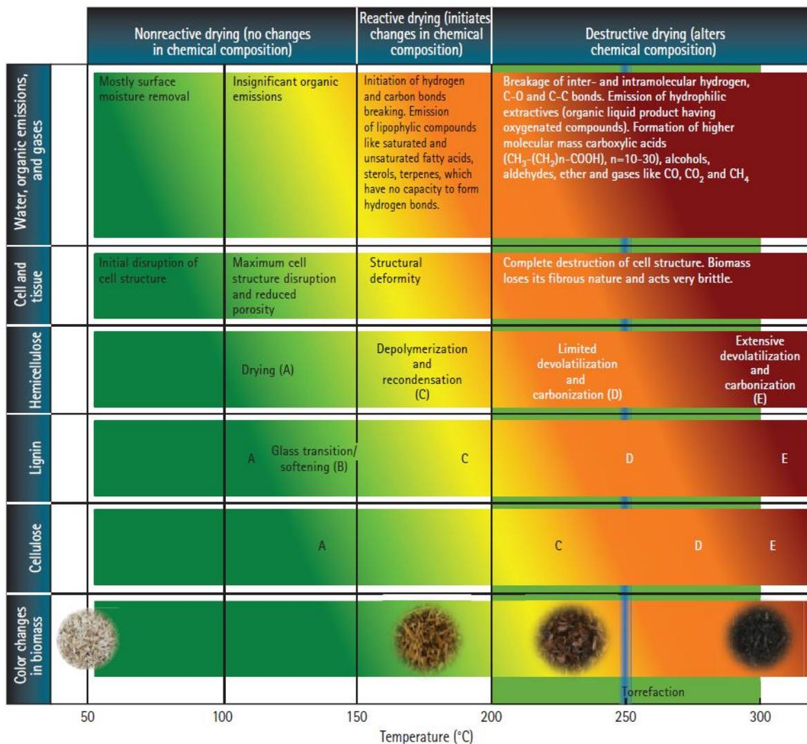
Figure 2. Structural, chemical, and color changes in lignocellulosic biomass during torrefaction. A: Drying, B: Softening/Glass transition, C: Depolymerization and recondensation, D: Limited devolatilization and carbonization, E: Extensive devolatilization and carbonization.
