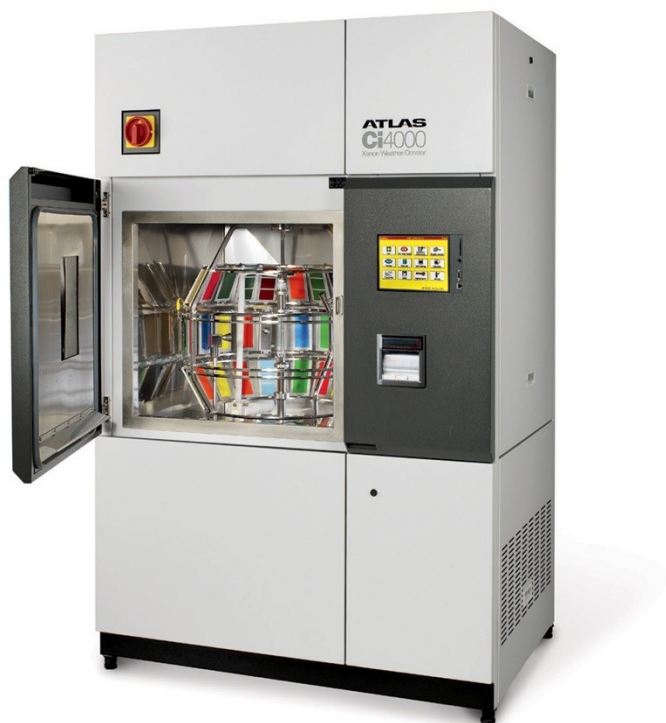
FIGUR 4.4: WEATHER-OMETER STAND ATLAS Ci4000
