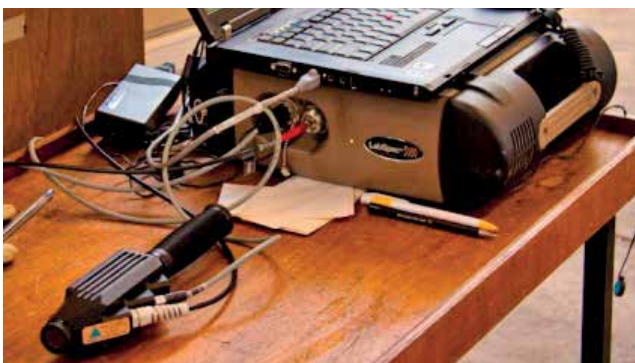
Figure 1. The ASD Labspec 5000 NIR spectrometer (left), the high intensity contact probe (centre) and application to a slice of lamb M. longissimus lumborum
