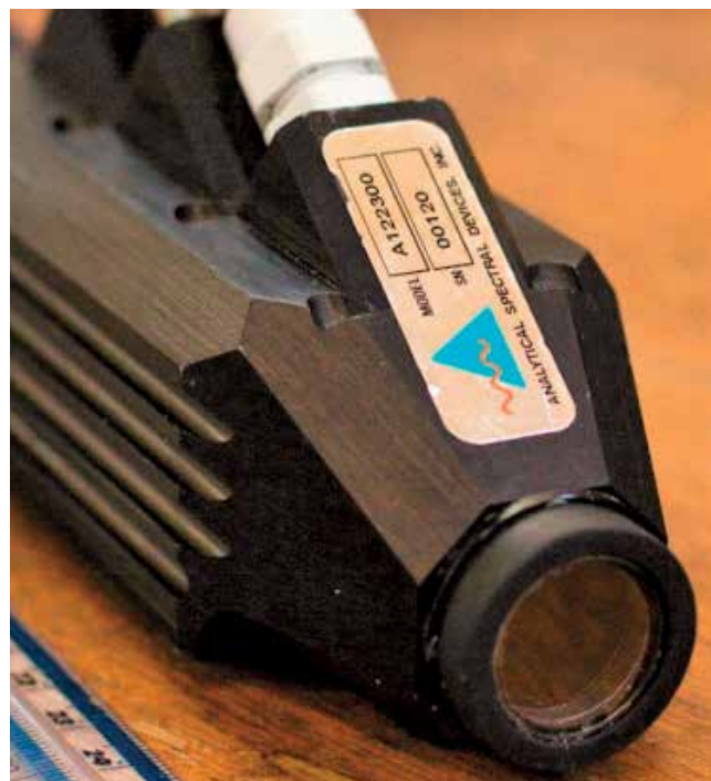
Figure 1. The ASD Labspec 5000 NIR spectrometer (left), the high intensity contact probe (centre) and application to a slice of lamb M. longissimus lumborum
