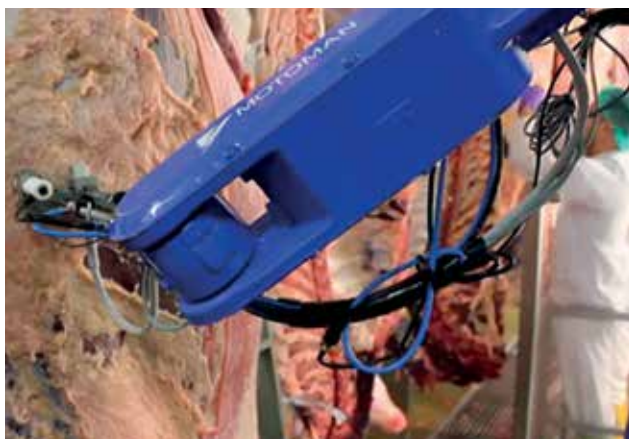
Figure 1. Autonomous robotic arm concept applying probes on-line to carcass line
