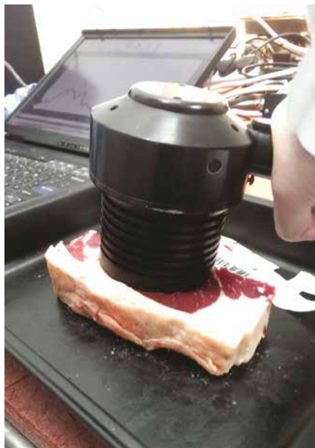
Figure 2. The NIRS system showing the measuring head applied to an excised M. longissimus thoracis steak.
