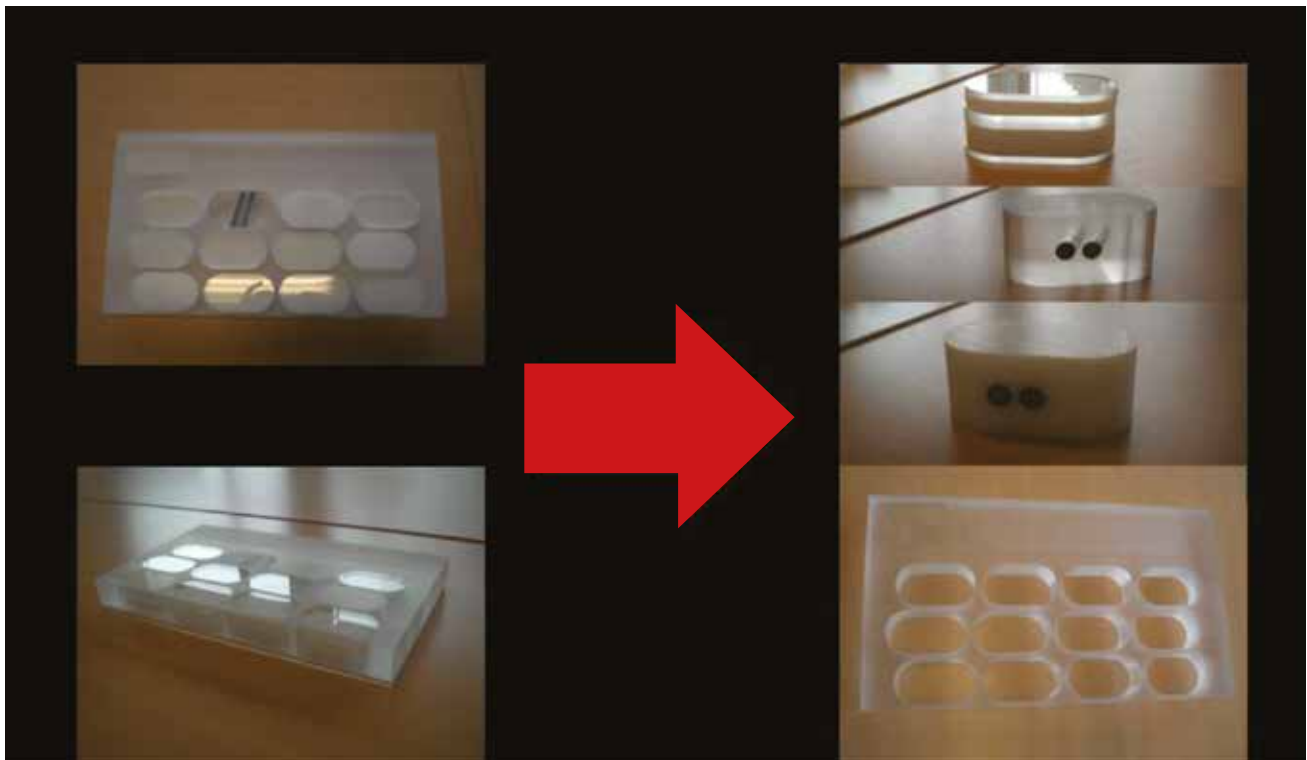
Figure 1. The belly phantom. One of the members of the belly phantom set assembled (left) and dismantled (right). The different members of PE (white), PVC (black) and PMMA (clear) are easily distinguishable. Before assembly the volume determination of the three polymers is made using a pycnometer.
