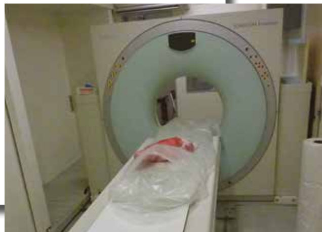
Figure 1. CT Scanning pork joints
