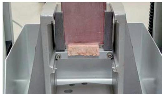
Figure 12: SSF shearing on a universal testing machine. From Shackelford et al. (2009).
