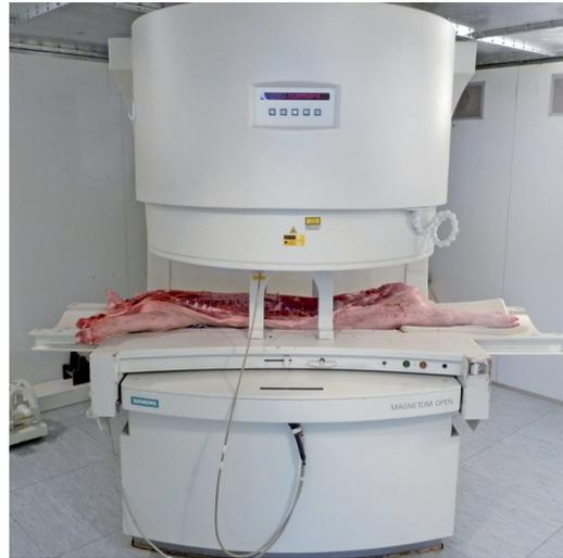
Figure 3: Pig carcass evaluated with a MRI equipment (photo courtesy of Armin Scholz, Ludwig Maximilian University of Munich).
