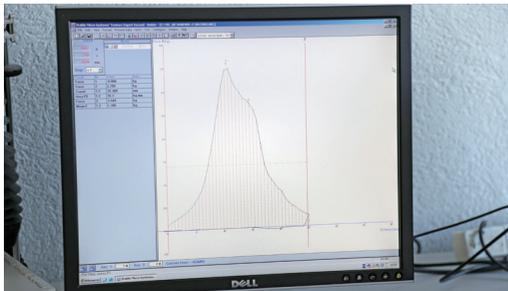
Figure 6: Force deformation curve. The peak force (maximum peak, number 3) is recorded here as kgf.
