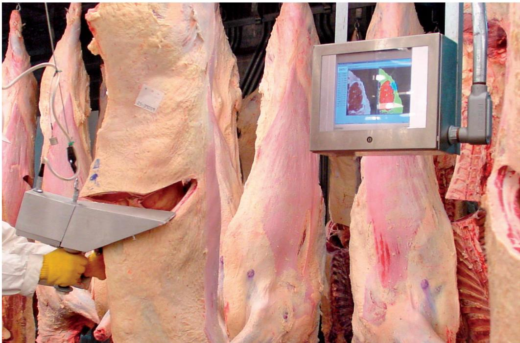
Figure 5: Beef loin image analysis to determine quality characteristics (photo courtesy of e+V Technology GmbH, Oranienburg, Germany).
