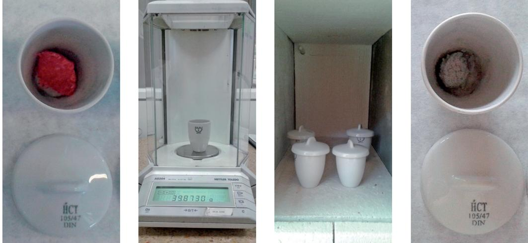
Figure 4: Ash evaluation process, from left to right, fresh sample, weighing, muffle oven and ash.
