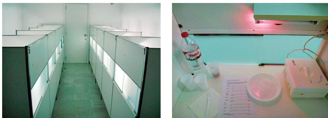
Figure 1: Sensory room with 10 booths (left) and detail of a prepared booth with red light (right).
