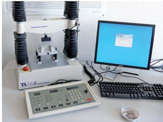
Figure 4: Electric testing machine fitted with a Warner-Bratzler shear blade.
