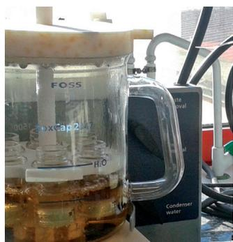
Figure 1: Acid hydrolysis process.
