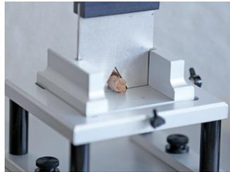
Figure 5: Performing a WB shear force measurement with an electric testing machine fitted with a Warner-Bratzler shear blade.
