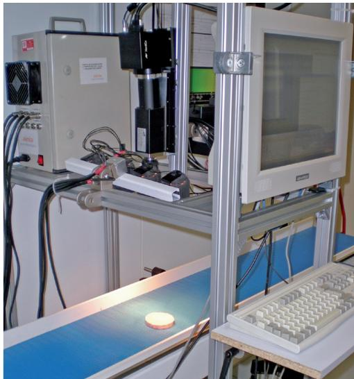
Figure 7: Hyperspectral analysis measuring a hamburger (photo courtesy of Ricardo Diaz, AINIA, Spain).
