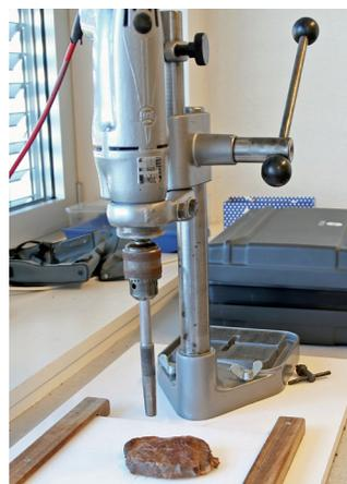
Figure 2: Electric drill press with cork borer attached.
