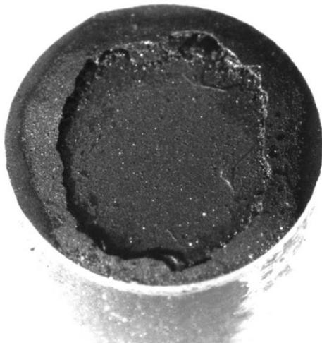
Figure 9: Photograph of the pole face of a magnetized NdFeB cylinder after 1 day of free corrosion in 0,005M H<sub>2</sub>SO<sub>4</sub>[3].
