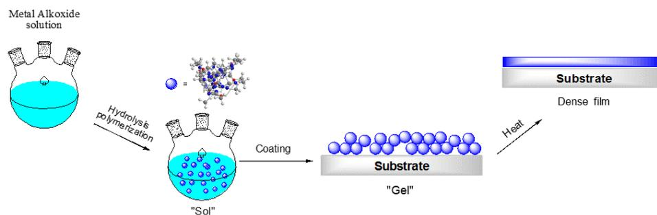
Figure 1: Overview of the coating synthesis procedure. Blue spheres; metal-oxo particles. After heating a dense coating is formed
