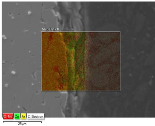
Figure 15 – Zn-coating in SEM at 10000x zoom with EDX
