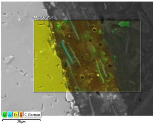
Figure 33 – Teflon-coating in SEM at 10000x zoom with EDX.
