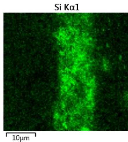
Figure 29 – EDS mapping of the Black Epoxy-coating, showing the presence of different atoms at 10000x zoom.
