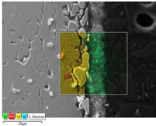
Figure 27 – Black Epoxy-coating in SEM at 10000x zoom with EDX.
