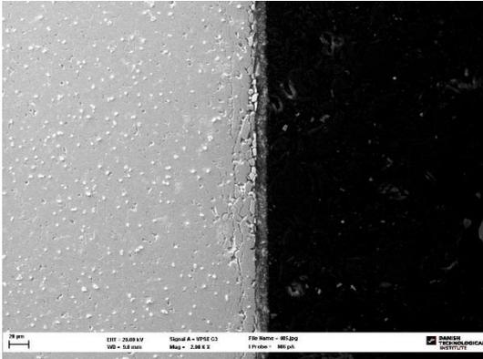
Figure 25 – Black Epoxy-coating in SEM at 2000x zoom.
