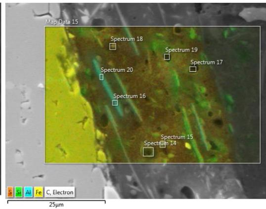
Figure 34 – Teflon-coating in SEM at 15000x zoom with EDX.
