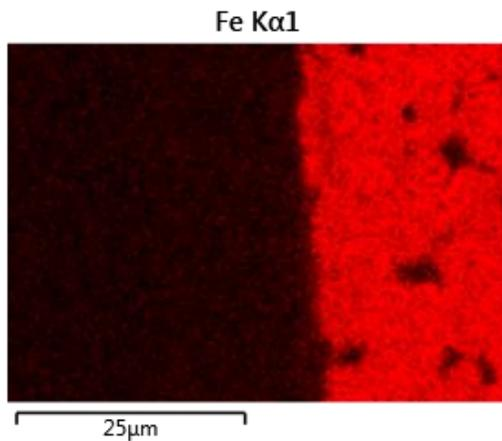
Figure 40 – EDX mapping of the Teflon-coating, showing the presence of different atoms at 10000x zoom.
