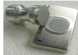
Figure 6 - Detachment between coating and magnet.
