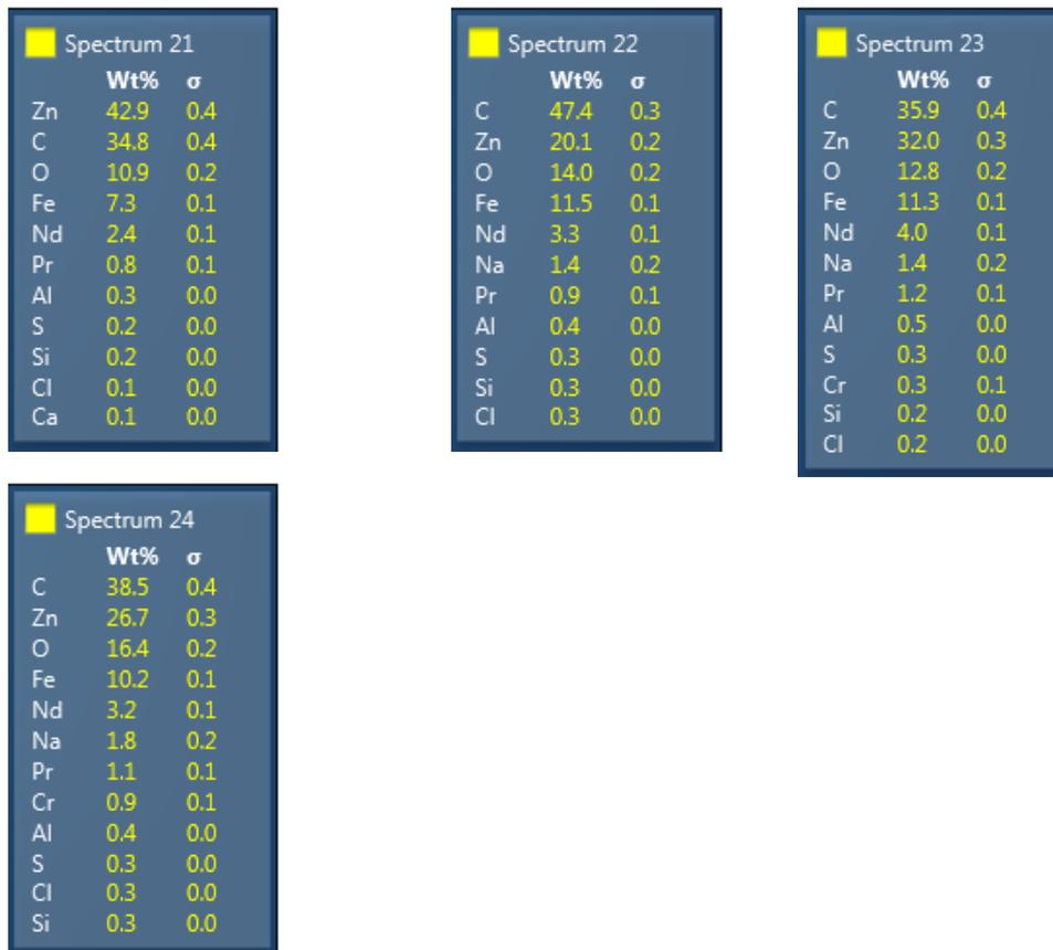
Figure 24 – Point analysis and mapping summary of EDX at 15000x, areas can be found in Figure 2223.
