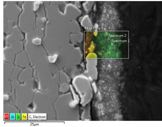
Figure 28 – Black Epoxy-coating in SEM at 15000x zoom with EDX.
