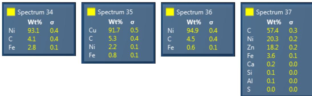
Figure 12 – Point analysis and mapping summary of EDX at 15000x, areas can be found in Figure 109.
