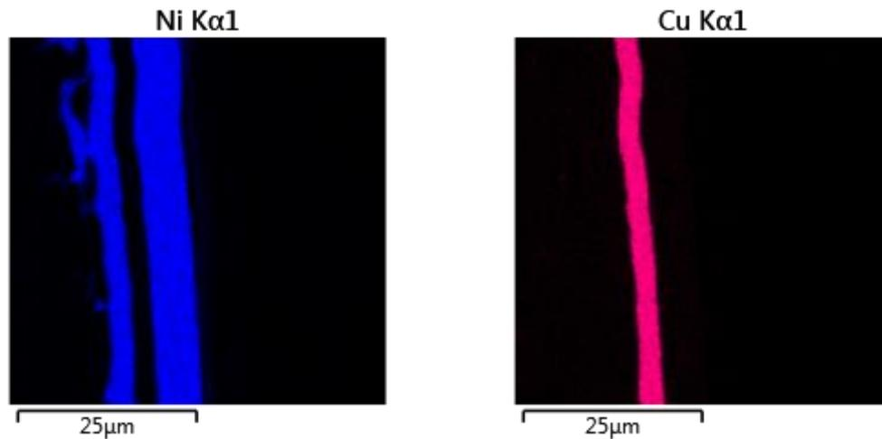
Figure 11 – EDX mapping of the NiCuNi-coating, showing the presence of different atoms at 10000x zoom.
