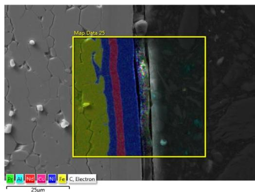
Figure 9 – NiCuNi-coating in SEM at 10000x zoom with EDX.
