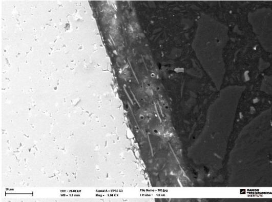
Figure 32 – Teflon-coating in SEM at 5000x zoom.
