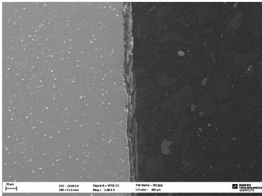
Figure 13 – Zn-coating in SEM at 2000x zoom.
