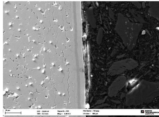
Figure 8 – NiCuNi-coating in SEM at 5000x zoom.
