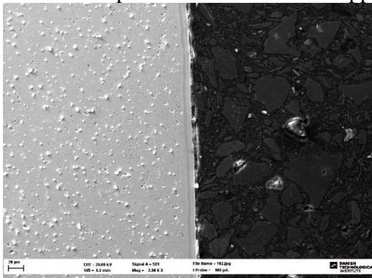
Figure 7 – NiCuNi-coating in SEM at 2000x zoom.
