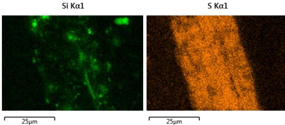
Figure 35 – EDX mapping of the Teflon-coating, showing the presence of different atoms at 10000x zoom.
