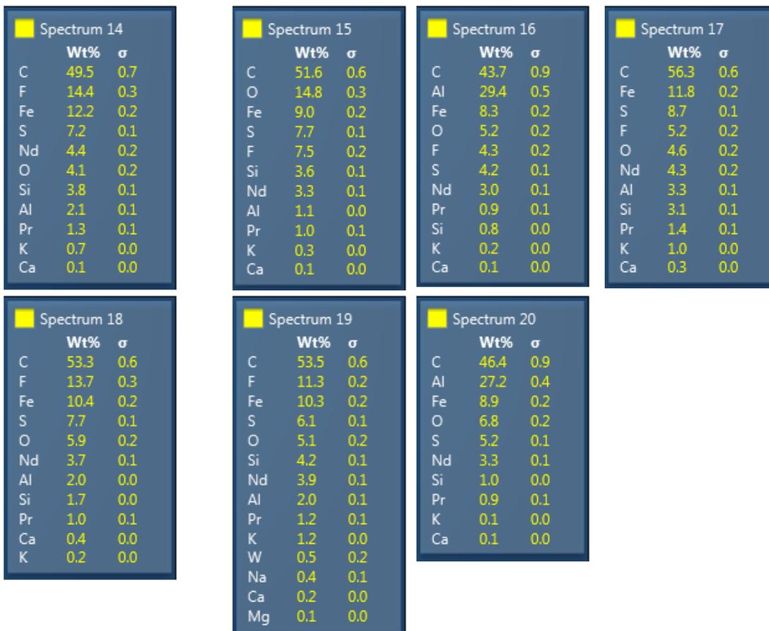
Figure 36 – Point analysis of EDX at 15000x, areas can be found in Figure 344.
