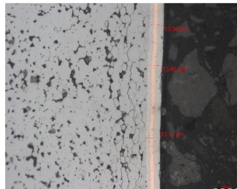
Figure 3: LOM picture of the surface of the Ni-CuNi coating
