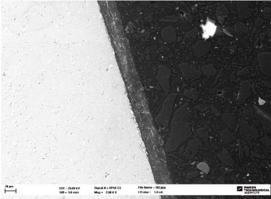
Figure 31 – Teflon-coating in SEM at 2000x zoom.
