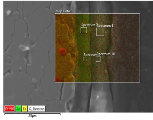
Figure 16 – Zn-coating in SEM at 15000x zoom with EDX.
