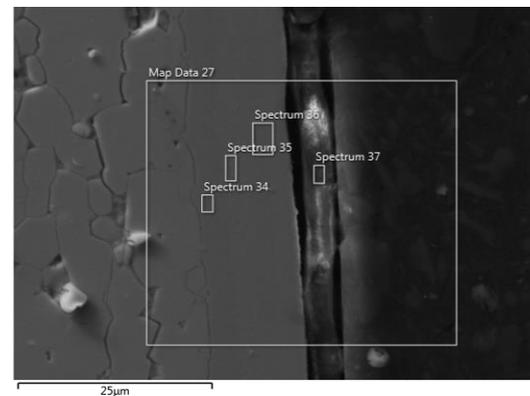
Figure 10 – NiCuNi-coating in SEM at 15000x zoom with EDX.
