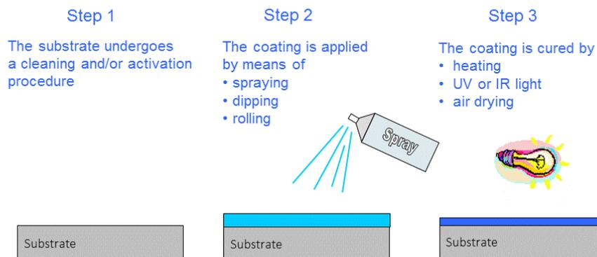
Figure 2: Overview of the coating process step by step
