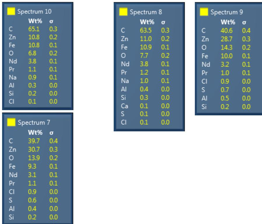
Figure 18 – Point analysis and mapping summary of EDX at 15000x, areas can be found in Figure 166.
