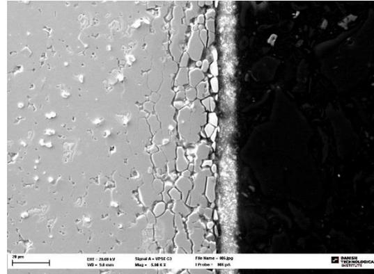
Figure 26 – Black Epoxy-coating in SEM at 5000x zoom.
