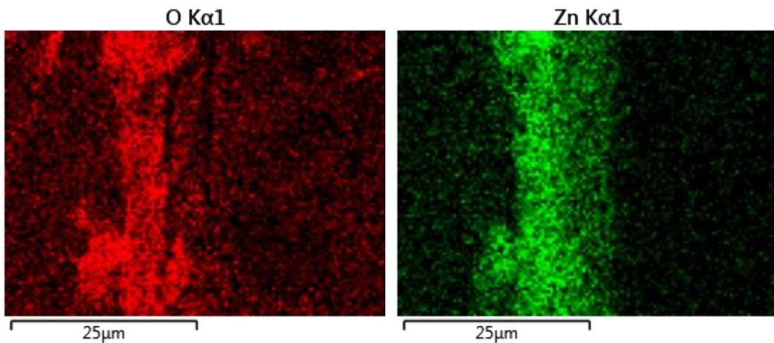
Figure 17 - EDX mapping of the Zn-coating, showing the presence of different atoms at 10000x zoom.
