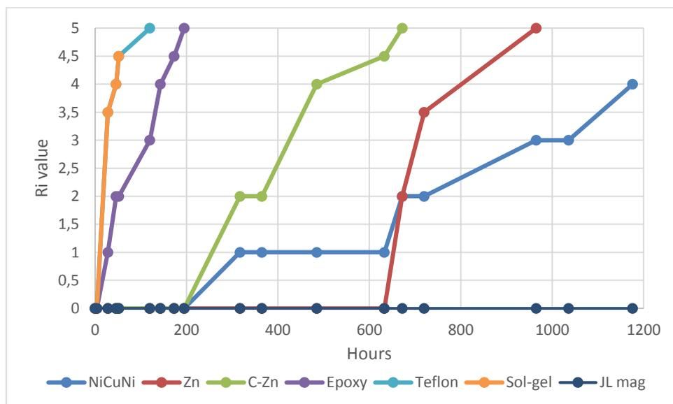
Figure 4 – Salt spray test of the samples graded according to ISO 4628-3:2003.
