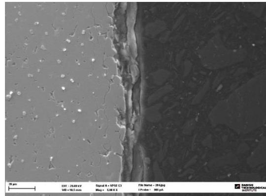
Figure 14 – Zn-coating in SEM at 5000x zoom.
