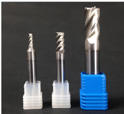
Tools coated with the new TiB 2 coating
