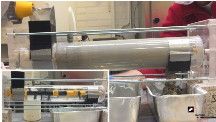
Functionally-graded concrete sample
