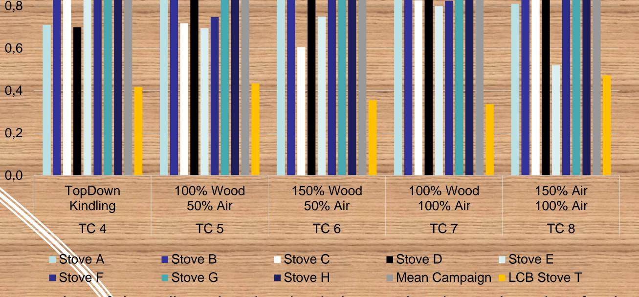
An overview of the collected and emitted elemental and organic carbon for the eight stoves, a combined mean from the campaign and the produced LCB Stove T for the different test cycles (TC) of wood quantities and air supply settings.
