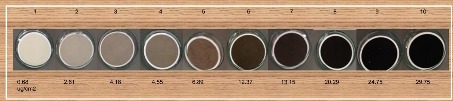
The measurement campaign revealed a correlation between the analysed and measured elemental carbon and the color from the collected particulate mass.
