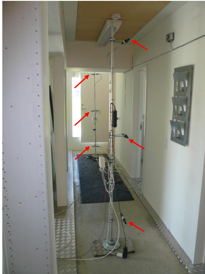
Figure 4.3. The stands with three combined temperature and rh sensors (at the arrows) in the aisle.
