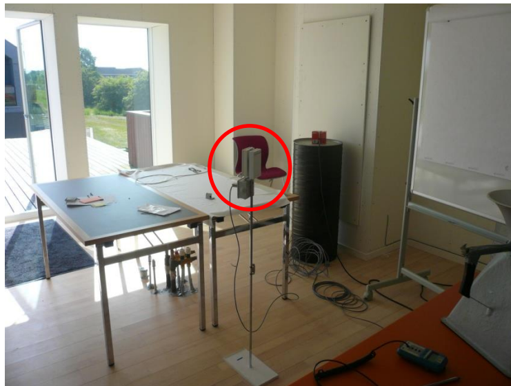
Figure 4.6. The Vaisala CO 2 sensor and Vaisala temperature/rh sensor in the kitchen on the first floor.
