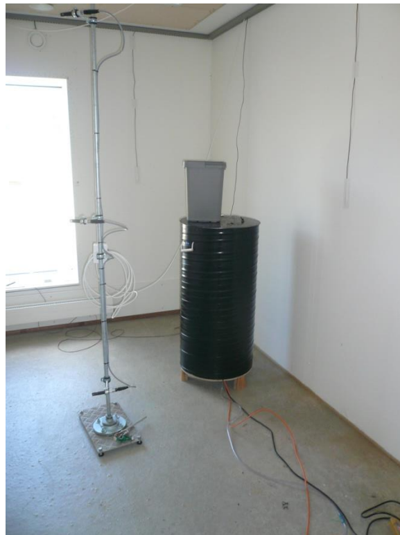
Figure 3.1. An artificial person in the form of a barrel and a bucket with water for the humidifier. The artificial persons were supplied with CO 2 from a common gas cylinder through plastic tubes.
