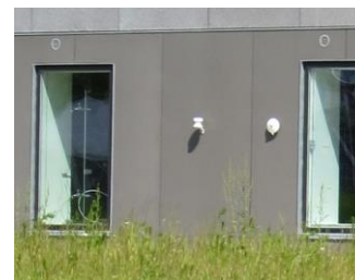
Pyranometer and temperature sensor at the south wall of EnergyFlexLab.
