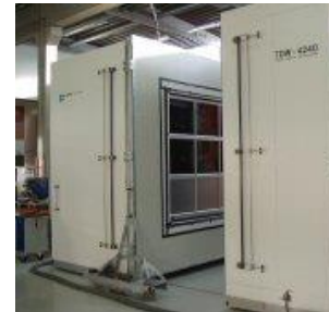
Test of building components in hot box.
