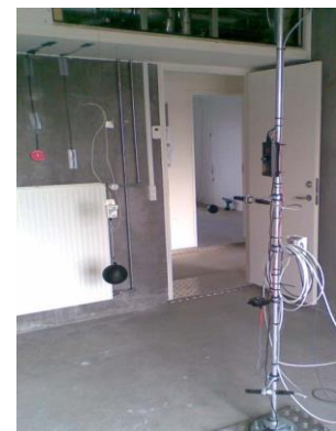
Air, globe and surface temperature sensors, humidity sensors, lux sensor and heat flux sensor in one side-by-side room in EnergyFlexLab.
