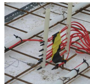
Embedded temperature sensors in the floor of one of the side-by-side test rooms in EnergyFlexLab before concrete was poured in.
