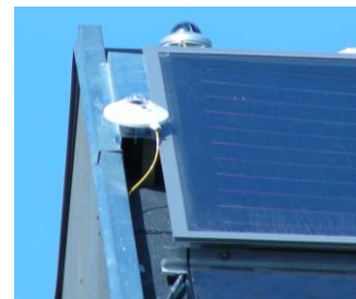
Pyranometers and pyrgometer at the roof of EnergyFlexLab.
