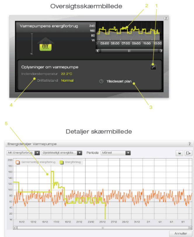
Figure 6. Shows the HP overview screen (top) and the HP energy consumption comparison graph (bottom).
