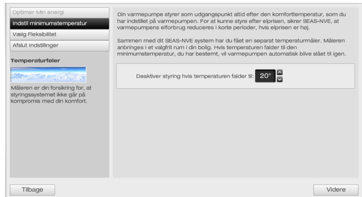
Figure 3. The screen for the comfort settings
