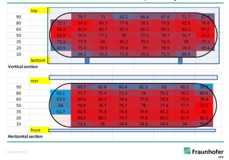
S107: measurement with thermocouple array
