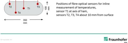
During heating, the temperature was measured in four places to ensure correct heating time and voltage.
