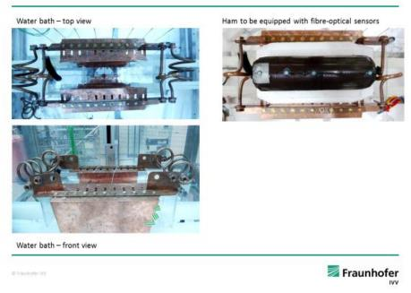
The pictures show the experimental set-up where one ham can be heated at a time.
