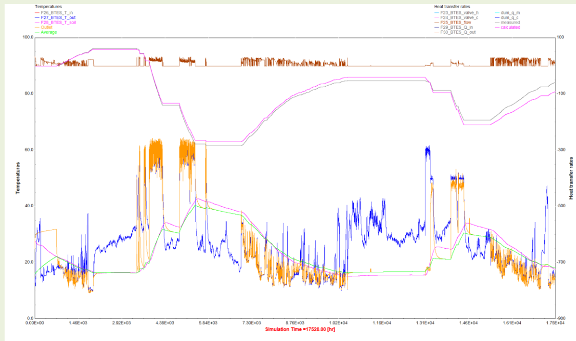
Figure 8: Comparison of measured and simulated values for 2014 and 2015. Brown = measured flow [ \text{m}^3/\text{h} ], blue = measured and orange = simulated outlet temperatures [ ^{\circ}\text{C} ], lower pink = measured and green = simulated storage temperatures [ ^{\circ}\text{C} ], and grey = measured and upper pink = simulated accumulated charging and discharging [MWh]. The first month is used for preheating the model, and is therefore not a part of the comparison.
