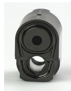
IBAD-DLC coated tool for forming the opening device on standard metal food cans. Due to the coating, the forming process can be performed without the use of lubricants for several months.
