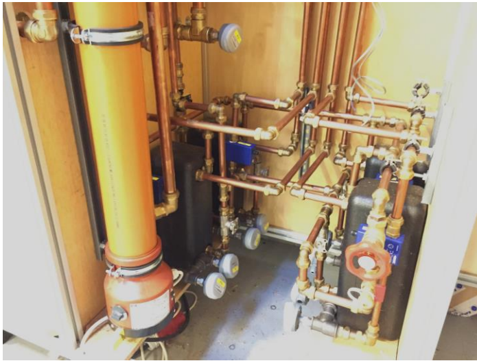
Figure 2.7. The heat emitting system of the test rig.
