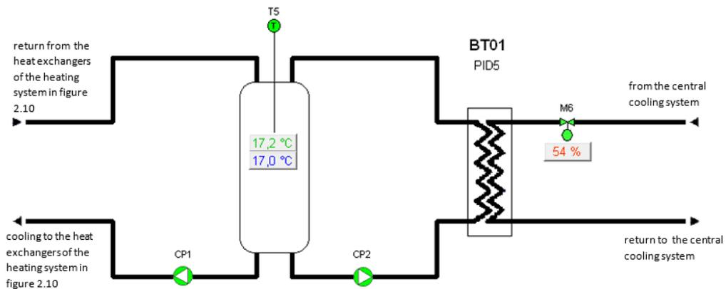
Figure 2.4. The BMS screen for viewing the controlling of the cooling system of the test rig.
