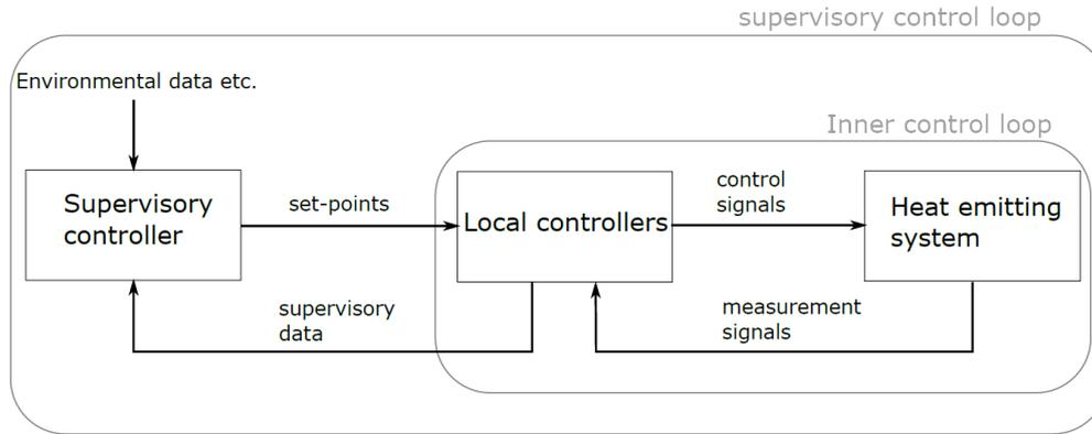
Figure 3.1. The two control loops of the investigated controller.
