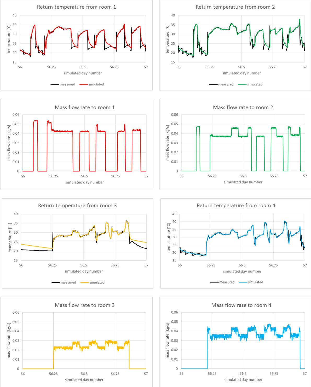
Figure 2.7. Simulated and measured return temperatures and measured mass flow rates for one day.
