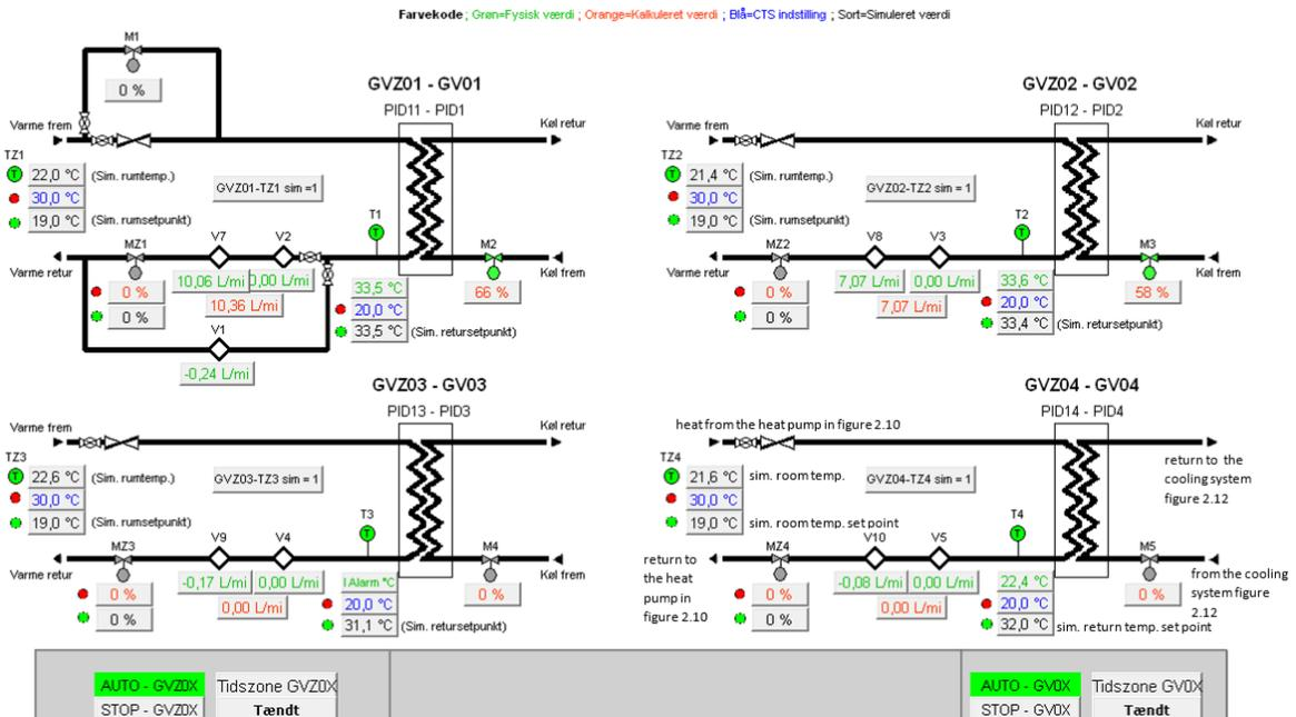
Figure 2.2. The BMS screen for viewing and controlling the four heating zones of the test rig.
