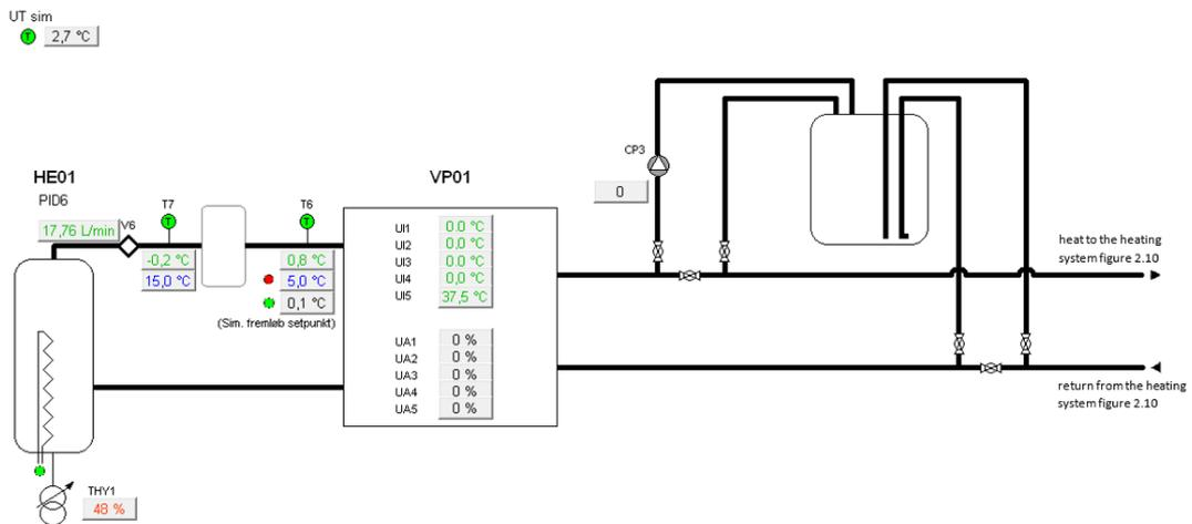
Figure 2.3. The BMS screen for viewing and controlling the heat pump and the brine side of the test rig.
