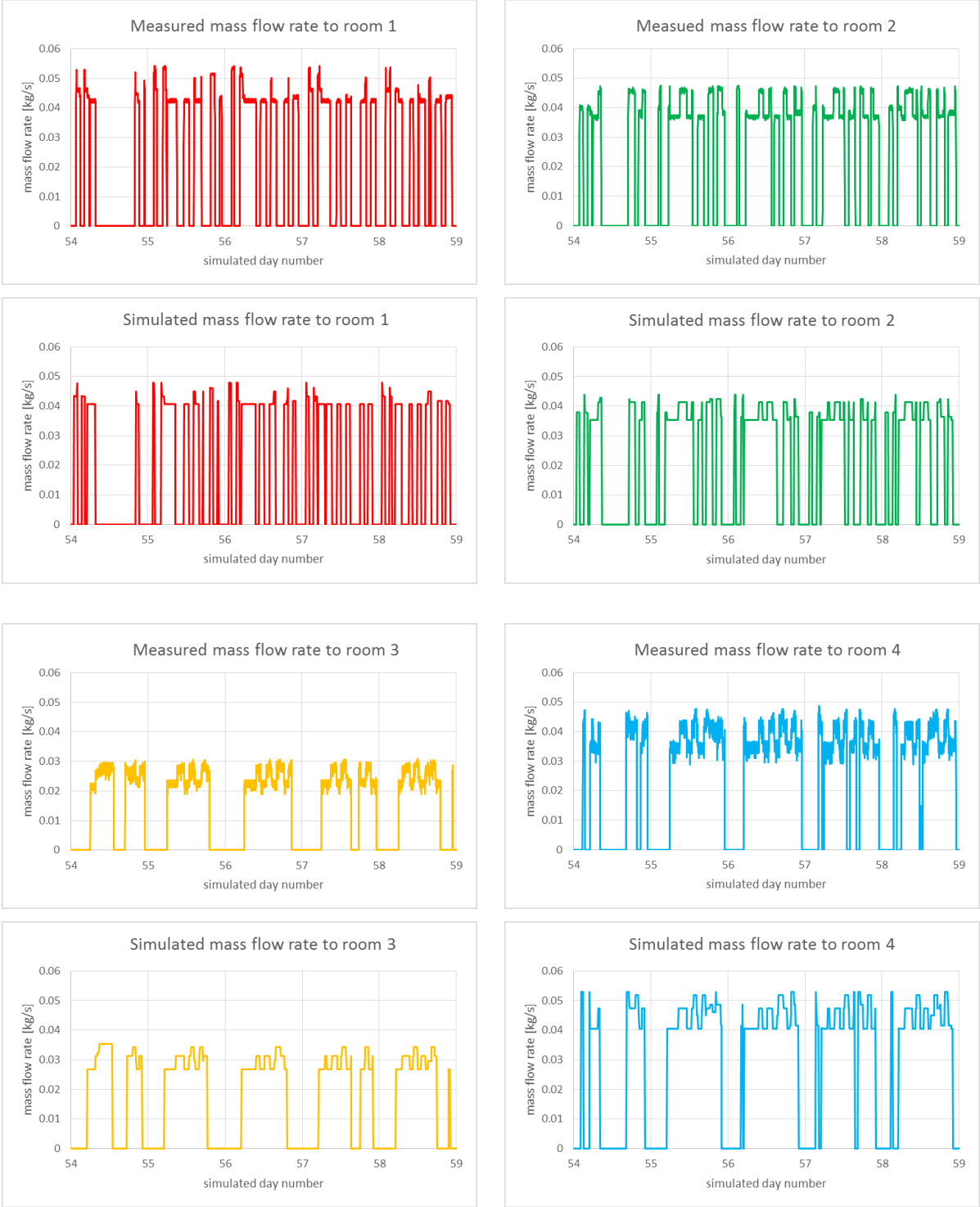
Figure 2.24. The measured and the simulated mass flow rates to the rooms. For room 1, one fourth of the flow rate and for room 2, one third of the flow rate.
