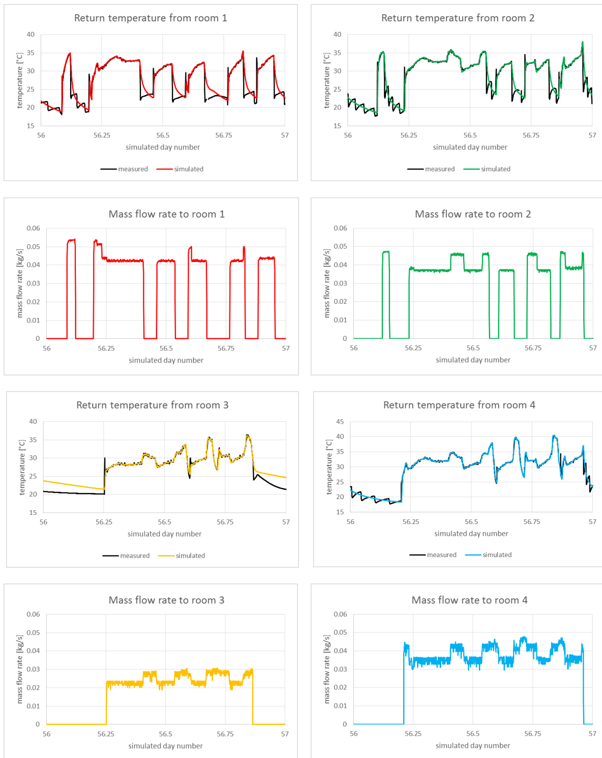
Figure 2.19. Simulated and measured return temperatures as well as measured mass flow rates for one day.
