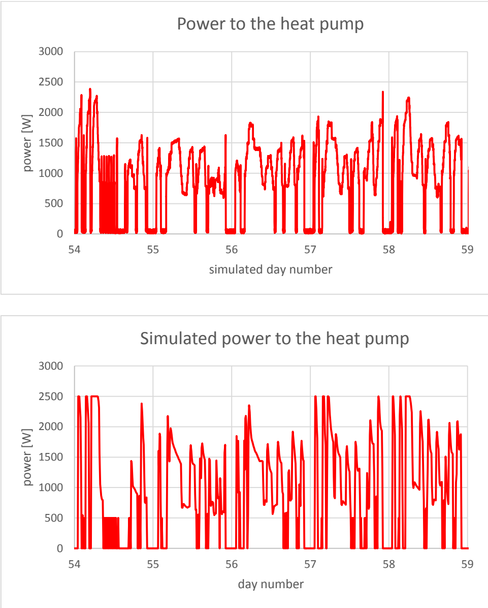
Figure 2.33. Power demand of the heat pump during the "warmest" period of the baseline test – measured on the test rig (top) and calculated by the annual simulation program (bottom).
