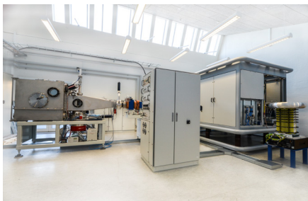
The new, high-current 1090 Danfysik accelerator currently being installed at the Tribology Centre, Danish Technological Institute, Aarhus.
