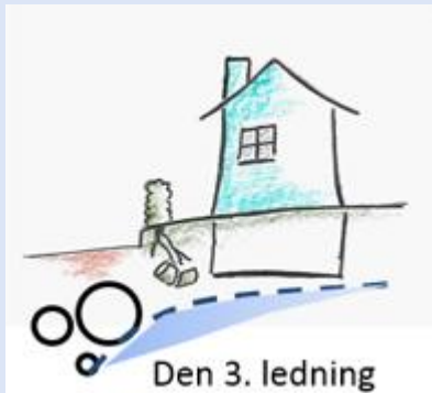
Figure 8: Horizontal subsurface drainage.
