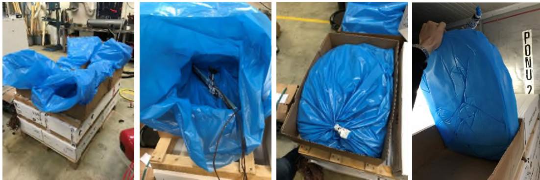
Figure 7: The construction of the measuring pallet. From the left: Water bags ready for water with thermocouples, in the middle in three different levels, finished water bag, and finally a frozen water bag.
