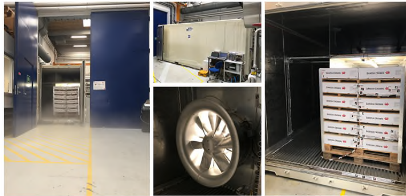
Figure 5: Selected images of the test setup at Danish Technological Institute. To the left a view into the open container. Middle upper is a side view of the container and the measuring equipment. Middle lower is the fan, and the one to the right is a view into the container looking at the third measuring pallet.
