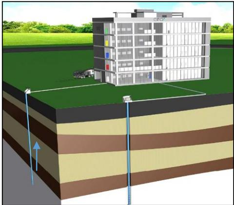
Groundwater is pumped from an aquifer through a well into the system and led to a heat exchanger setup through a pipeline
