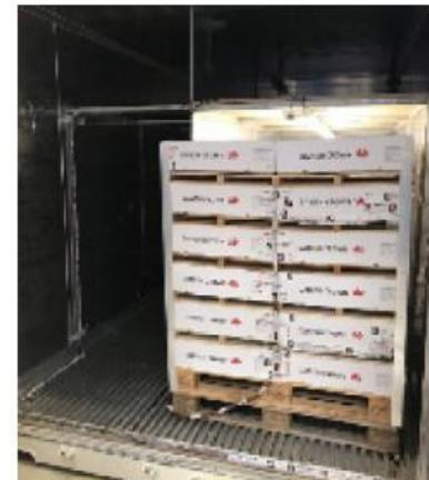
Figure 5: The third product pallet and return air channel
