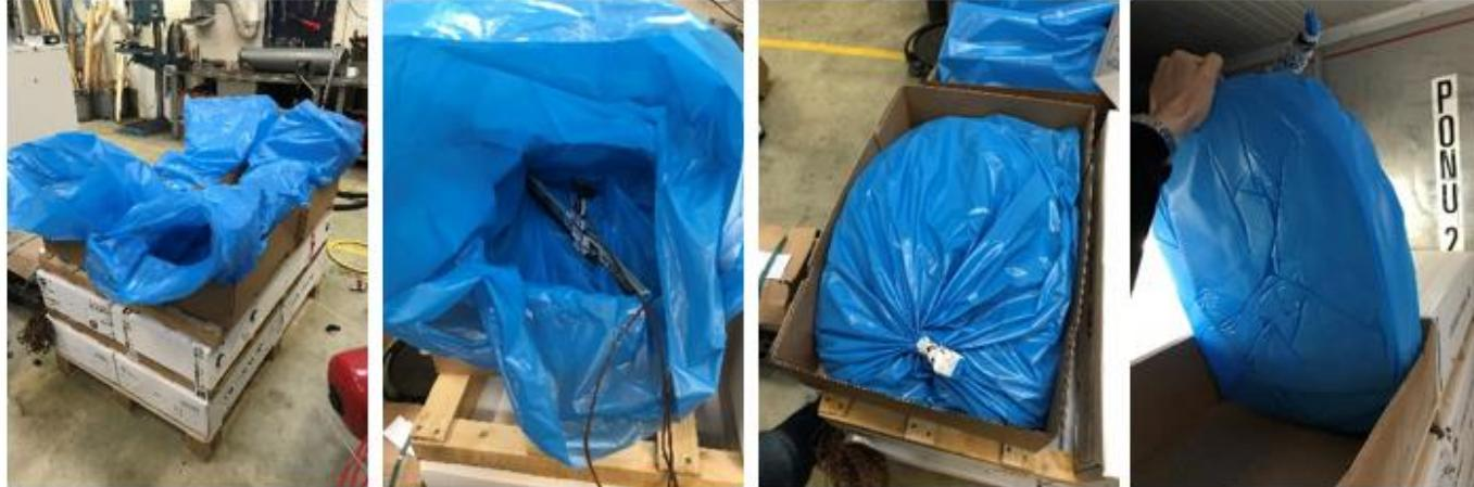
**Figure 8: The construction of the measuring pallet. From the left: Water bags ready for water with thermocouples, in the middle in three different levels, finished water bag, and finally a frozen water bag.**
